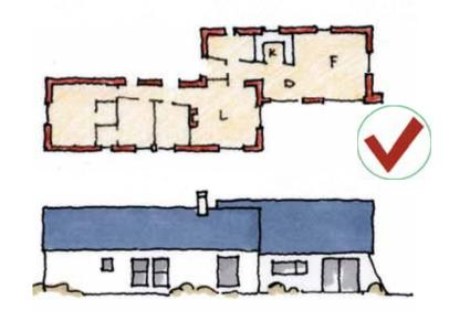
**NARROW PLAN -** plan facilitates window glazing options. Leads to more satisfactory ratio of glass to masonry. Greater freedom in composition.
