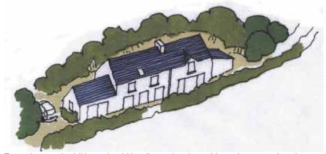
Extensions and additions should be directed to the gable end or rear elevation
