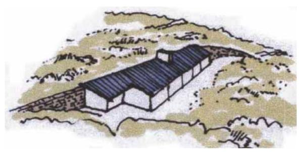
The narrow plan form reduces the need for an excavated platform The house elements are broken down and follow the contours
