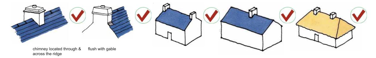
Chimney stacks add interest to a house and as a general principle for rural houses they should be located through and across the ridge. Where chimneys are located at gables, they should preferably be flush with the face of the wall, as is a feature characteristic across most of Cork. In East Cork, however, stout stacks built proud of the gable are a feature typical to the area.
