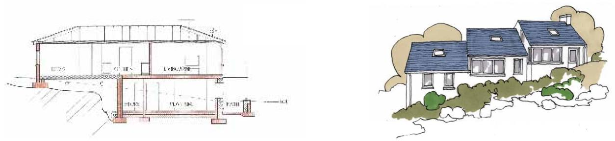
A slope can be accommodated without altering the ground, simply by changing the internal floor levels to suit. Seek a naturally flat site or cut into the hillside. Try to orientate the building with the contours to give an integrated appearance with the land, provide shelter and warmth, and reduce energy loss due to exposure.
