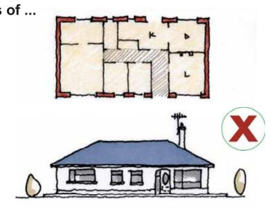
**DOUBLE ROOM DEEP PLAN** - typical plan layout with internal corridor places constraints which dictate the size and location of windows resulting in too much glass in relation to masonry.
