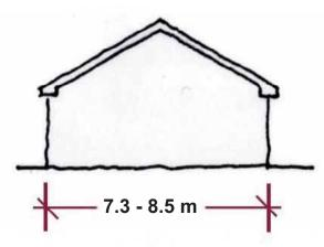
The 90's 'big house' - Double deep plan, bulky proportion, off centre chimney, shallow roof pitch, adorned frontages, mid-roof dormers, large roof spaces, cluttered finishes.
