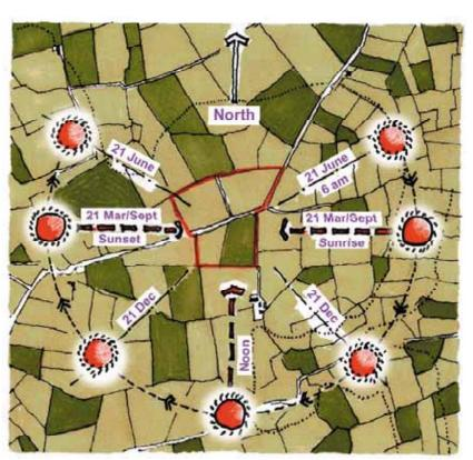
30% energy savings can be achieved if a house is orientated within 15° of south, providing its main living spaces are arranged to avail of the passive solar gains. Cork County Council's Energy Agency are able to provide free impartial advice on issues relating to energy efficiency when planning a site layout and designing a house. They can be contacted at:
