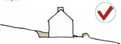
NARROW PLAN - Parallel with slope - narrow
