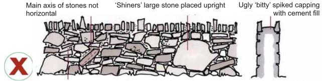
Large wide mortar joints flush with surface
