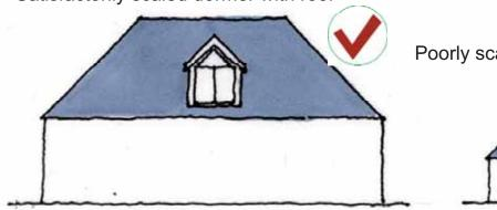
Poorly scaled dormer with roof
