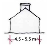
**The 70's bungalow**: Wide plan - dark central corridor, shallow pitched roof, horizontally proportioned openings, imported synthetic finishes.
