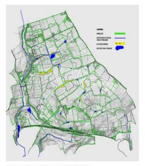
Figure 6.6 Proposed Swales, Detention Ponds and Filter Strips
