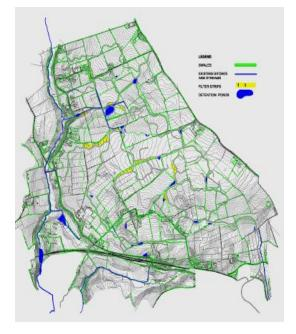
APPENDIX 2 Proposed Swales, Detention Ponds and Filter Strips
