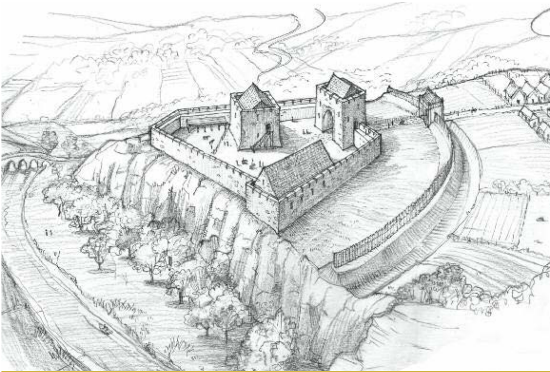
Reconstruction drawing of Glanworth castle as it would have looked c. 1300. The chamber-tower is at the centre of the enclosure, the gatehouse to the right and the hall in the foreground, incorporated into the curtain wall. The town is off to the right. Illustration by Rhoda Cronin.
