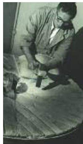
Neily O'Regan dressing a millstone at Howards Mill c.1960 ( Bridget and Michael Goulding).
