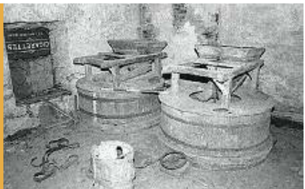
Two sets of millstones enclosed in wooden casing at Russagh, near Skibbereen, before it was renovated. (Cork Archaeological Survey, 1986).
