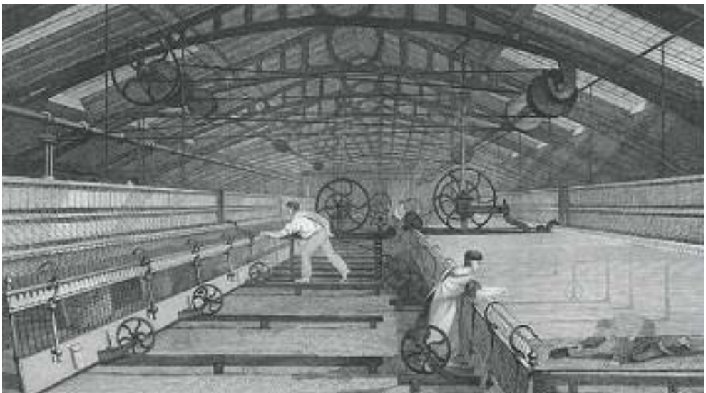
Mule spinning in a Lancashire cotton mill, around 1830.
