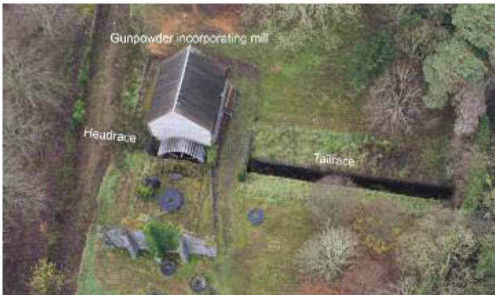
Head and tail race channels of gunpowder incorporating mill, Ballincollig Gunpowder Mills.
