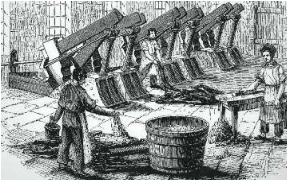
Fulling stocks at work in a nineteenth century woollen mill agitating the wool in the wooden trough. The power line is visible entering the mill, each turn of the power line turned the cam wheel and tripped the stock.
