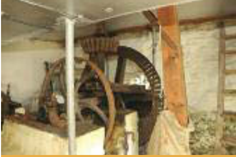
The mill basement with its gearing system. The cast iron bevelled pit wheel (which had wooden cogs), engaged the wallower which rotated the millstones overhead. The wooden chute directed the meal from the millstones into the meal bag.
