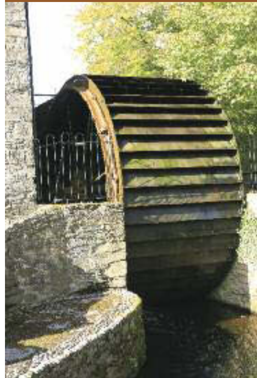
BELOW: High breastshot all-iron waterwheel at Bealick Mills, near Macroom.
