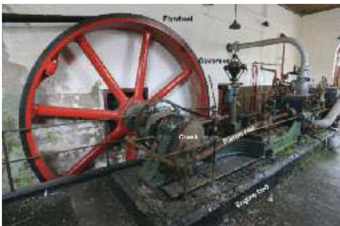
Horizontal textile mill engine at Orr's Mill, Benburb, County Tyrone.
