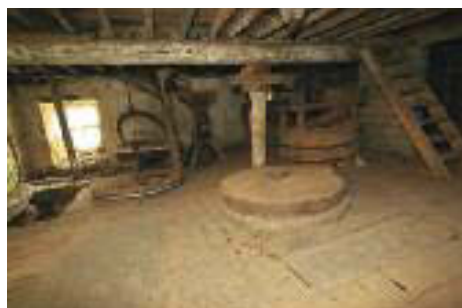
General view of millstone floor at Castleview Mills. The set of stones in the foreground are the sandstone shelling stones. The two sets at the rear are the French burr stones. The one on the right has its wooden box with a hopper set on top delivering the grain into the millstone. The runner stone on the left pair has been lifted by a crane and the stones are ready to be dressed.
