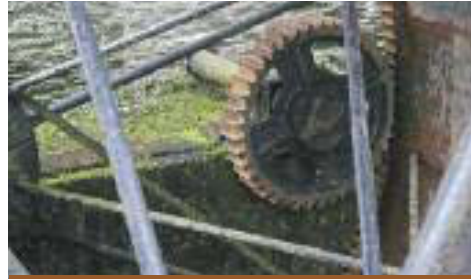
Bull nut engaging with segment gearing attached to the rim of the Suspension waterwheel at Bealick Mill.
