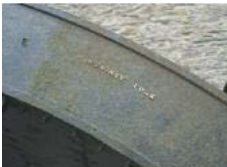
McSwiney's of Cork foundry stamp on the Bealick suspension waterwheel. This indicates that it must have been installed before 1860.
