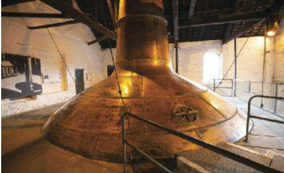
Main pot still at Midleton Distillery, installed in 1826 with a capacity of 31,648 gallons. This is reputedly the world's largest pot still.
