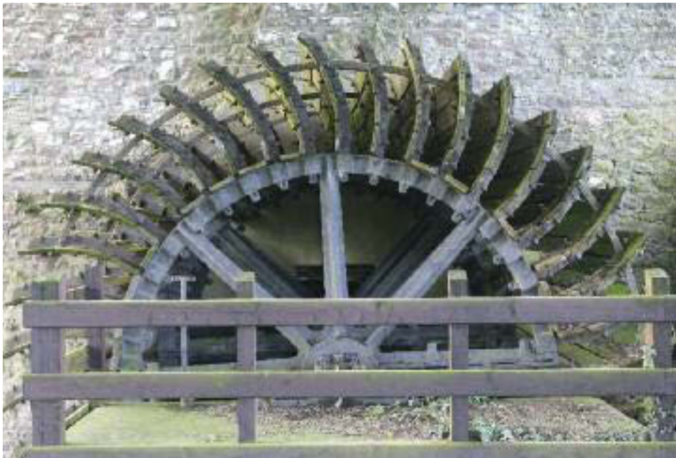
Poncelet advanced undershot waterwheel of c. 1860, at Glanworth Woollen Mill.
