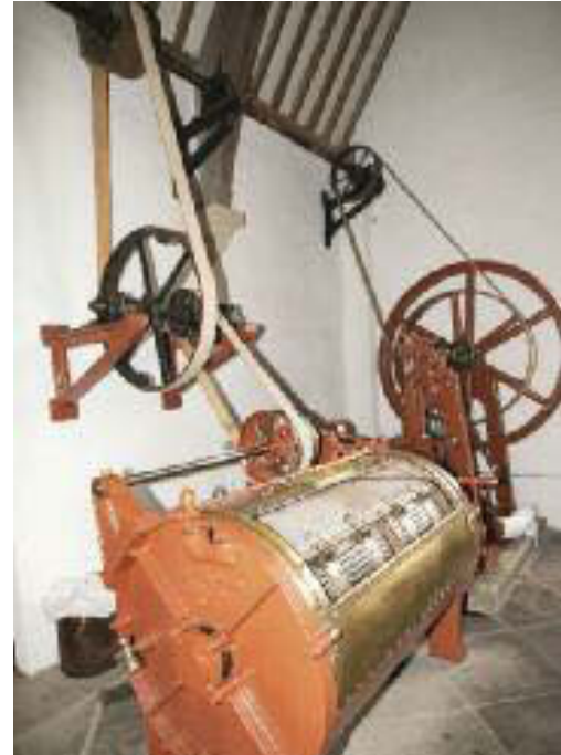
A-framed engine originally installed at Allman and Dowden's Brewery at Bandon, dating to the 1830, now on display at the Steam Museum Straffan, county Kildare. Note also the use of lineshafting and belt drives.
