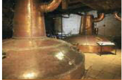
Low wines and feints stills, at Midleton Distillery, installed in 1949.
