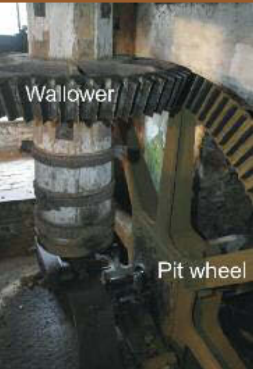
BELOW: Pit wheel and wallower gearing.
