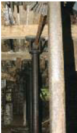
Nineteenth-century lineshafting in saw mill at Glenville.
