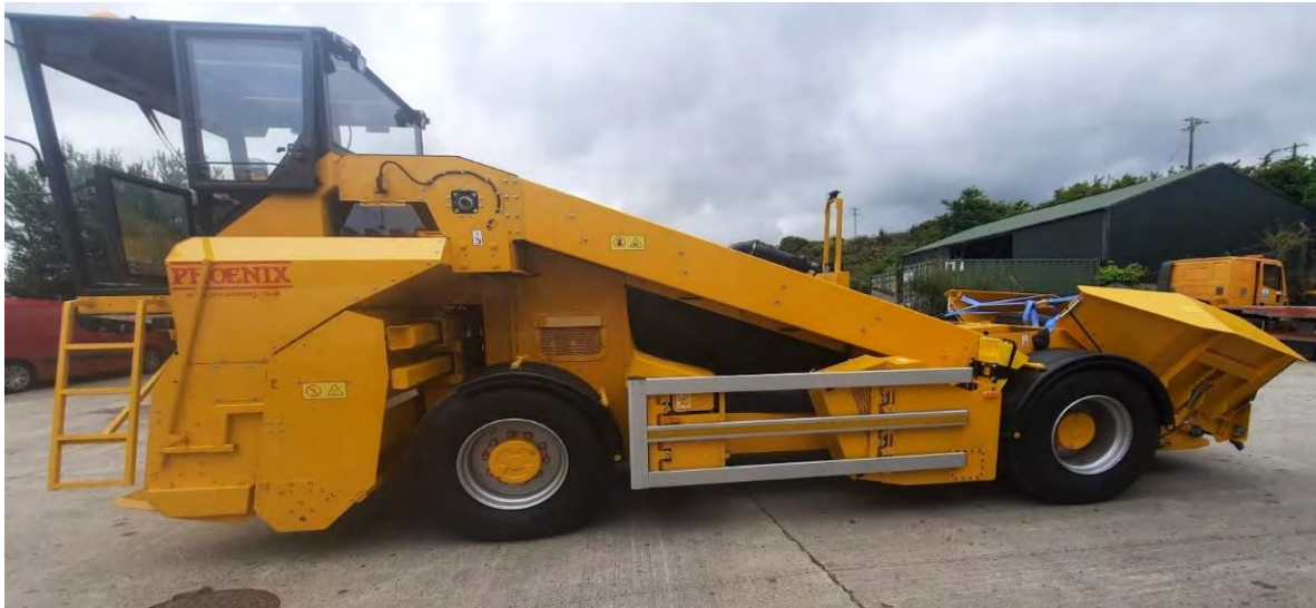
Chip spreaders – for road construction works, by direct labour – and to replace older machines
