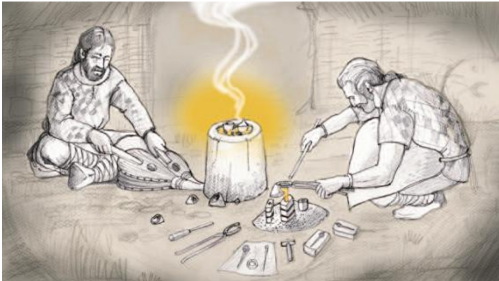
Artist impression of Early Christian metal workshop showing bronze being poured from a crucible into a bivalve mould. Drawing by Rhoda Cronin.
