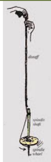
Diagram shows a woollen thread being spun using a spinning whorl and a spindle shaft. Drawing by Sheila Ronan.
