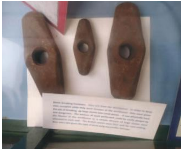
Stone breaking hammers from Clonakilty Workhouse, as exhibited in the West Cork Regional Museum, Clonakilty. Small broken stone was the main material used in road construction and in much demand in the 19th century.
