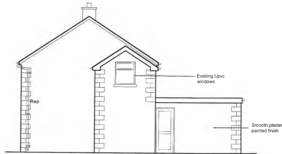
EXISTING NORTH ELEVATION
