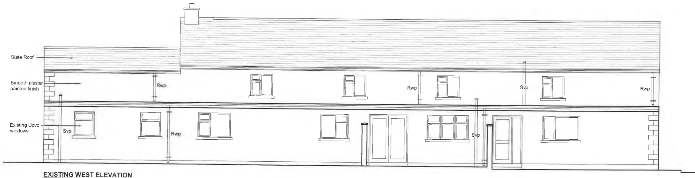
EXISTING WEST ELEVATION
