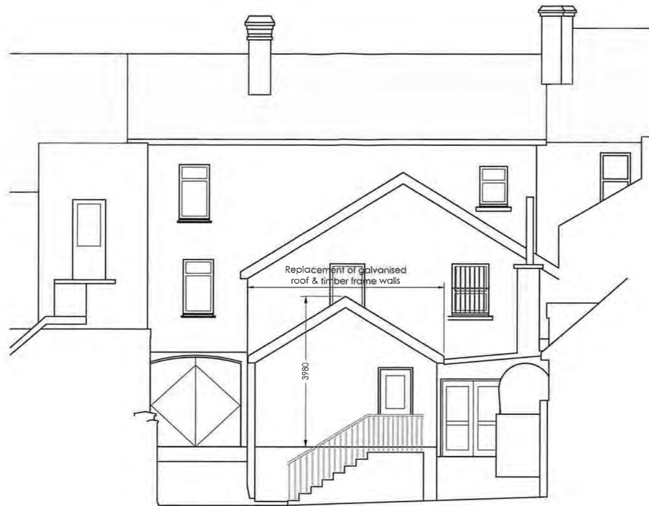
Proposed Rear Elevation ( East ) Scale : 1:100
