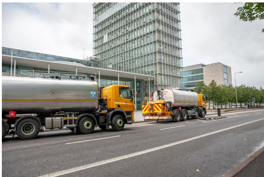
32 Tonne Tar Tank
