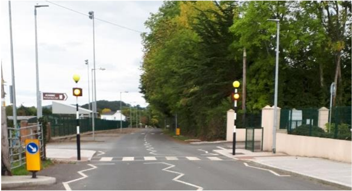
Low level lanterns located on both diagonals – preferred, or
