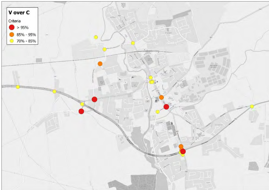
Figure 2 AM V/C Analysis – Rail Test Midleton
