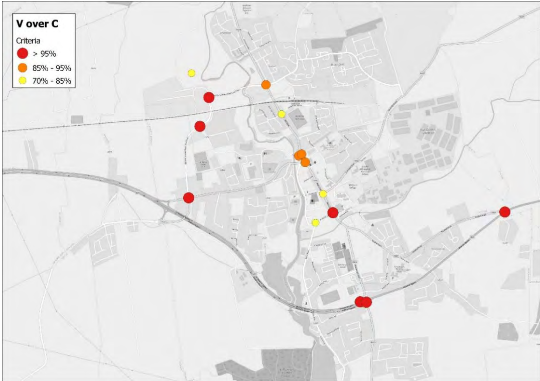
Figure 6 PM V/C Analysis – Rail Test Midleton
