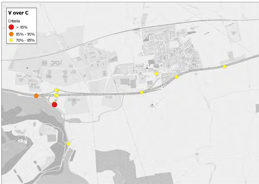
Figure 8-3 AM V/C Analysis – Do-Minimum Carrigtwohill
