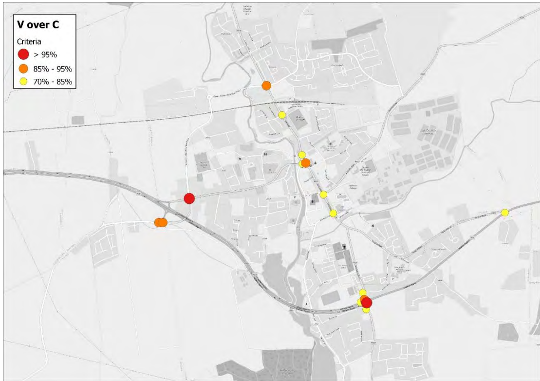
Figure 10 AM V/C Analysis – Rail Sensitivity Midleton
