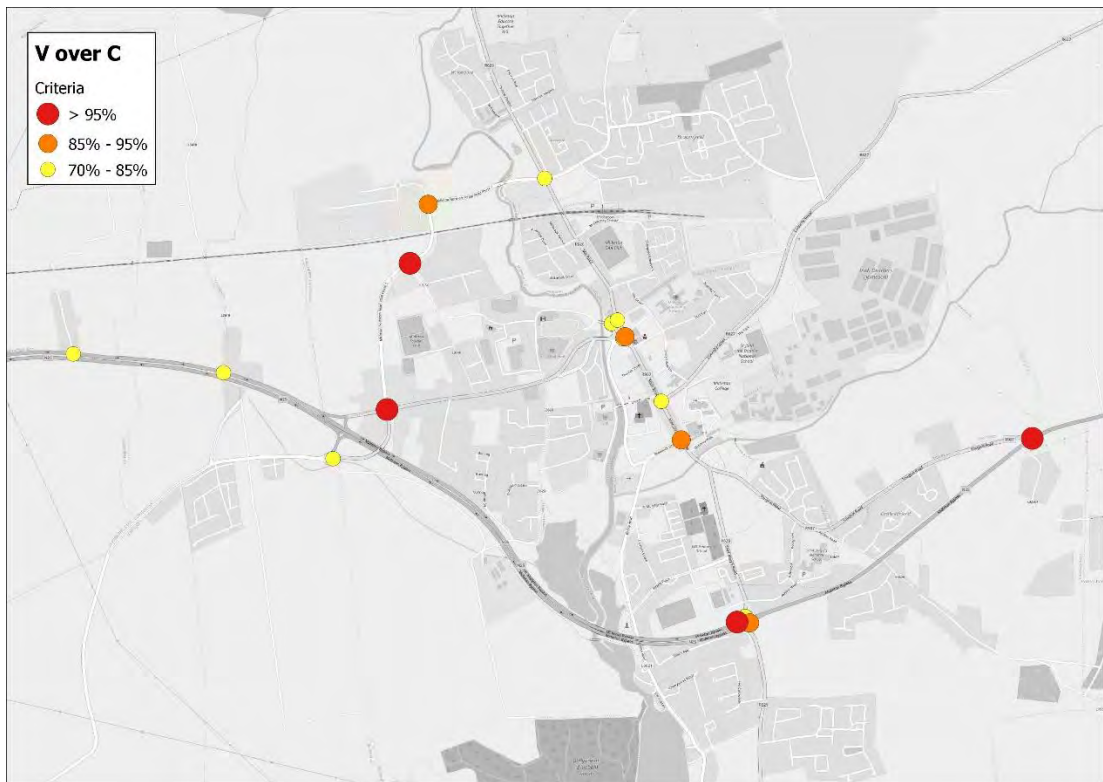
Figure 9-7 PM Peak (17:00 to 18:00) V/C Analysis – Do-Minimum Carrigtwohill
