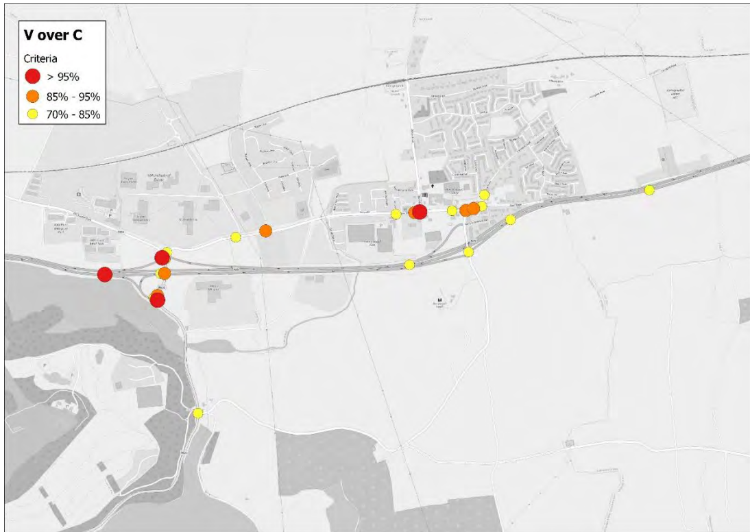
Figure 4 AM V/C Analysis – Rail Test Carrigtwohill
