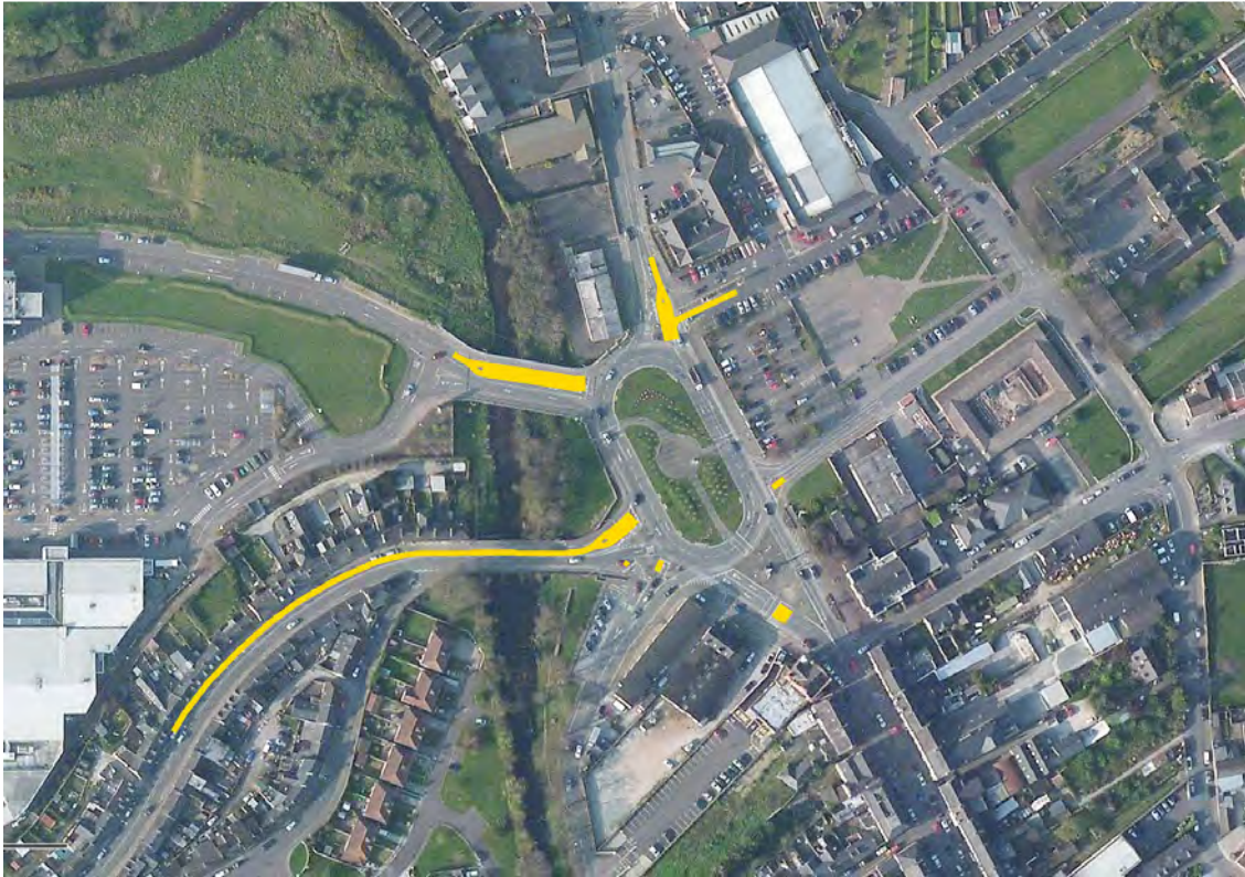
Figure 3-5 - Phase 1a Gyratory Average Queue with Right Turn Allowed at Knockgriffin
