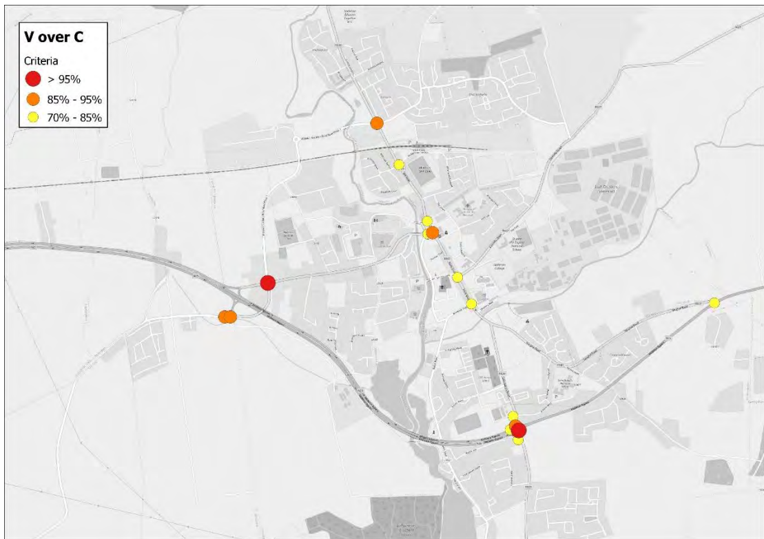
Figure 10 AM V/C Analysis – Rail Sensitivity Midleton
