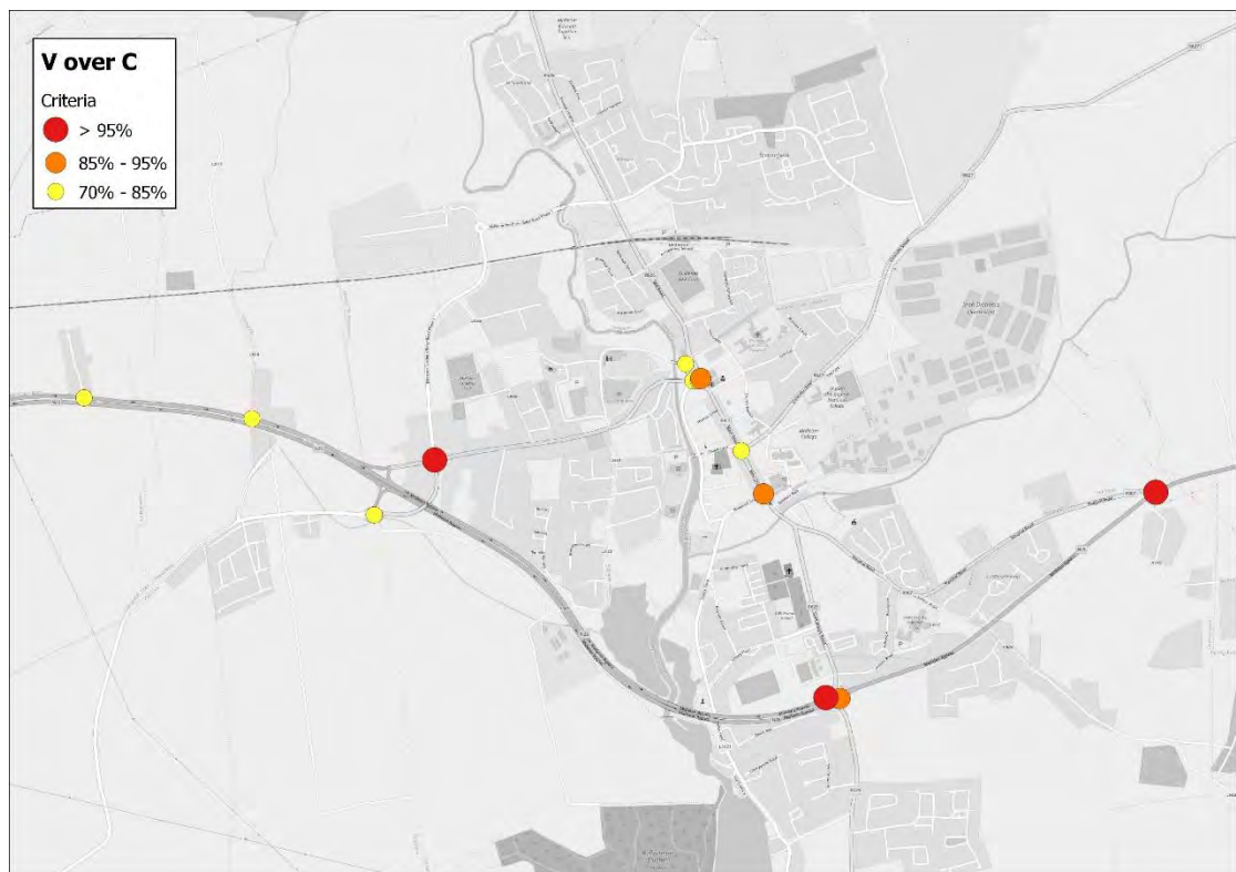
Figure 9-5 PM Peak (17:00 to 18:00) V/C Analysis – Do-Minimum Midleton
