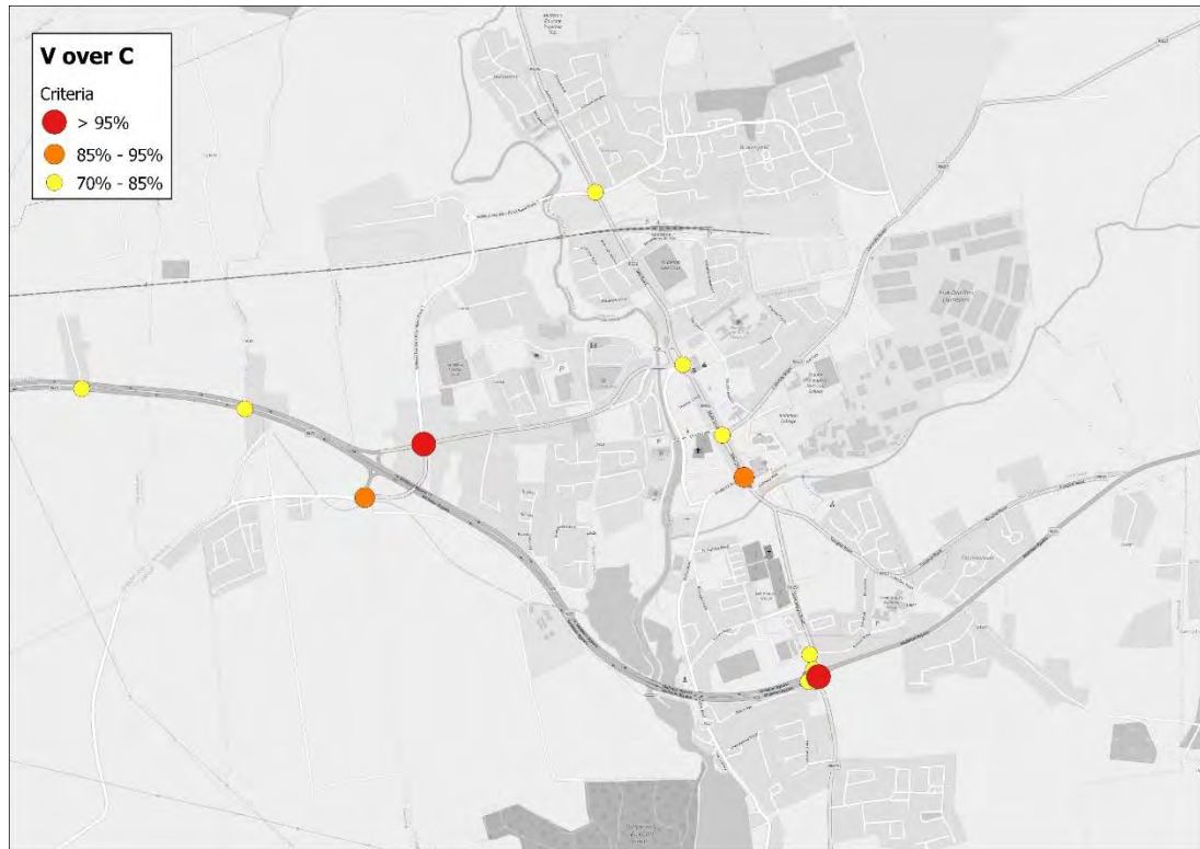
Figure 8-1 AM V/C Analysis – Do-Minimum Middleton
