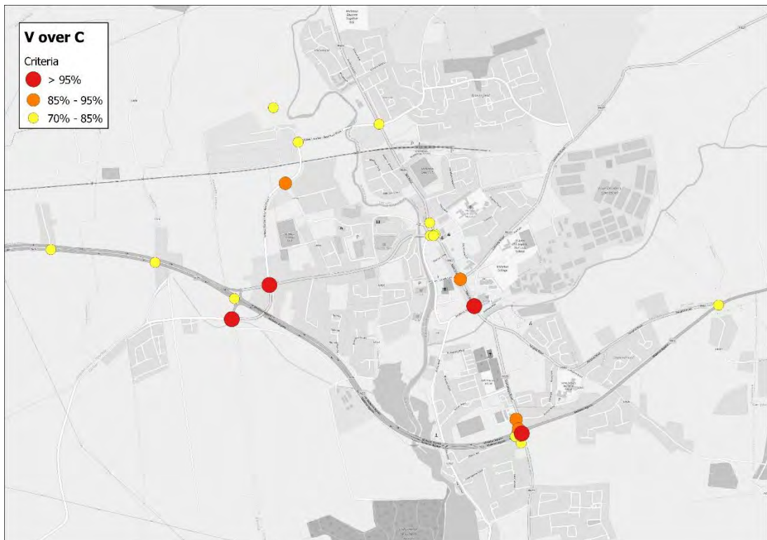
Figure 2 AM V/C Analysis – Rail Test Midleton
