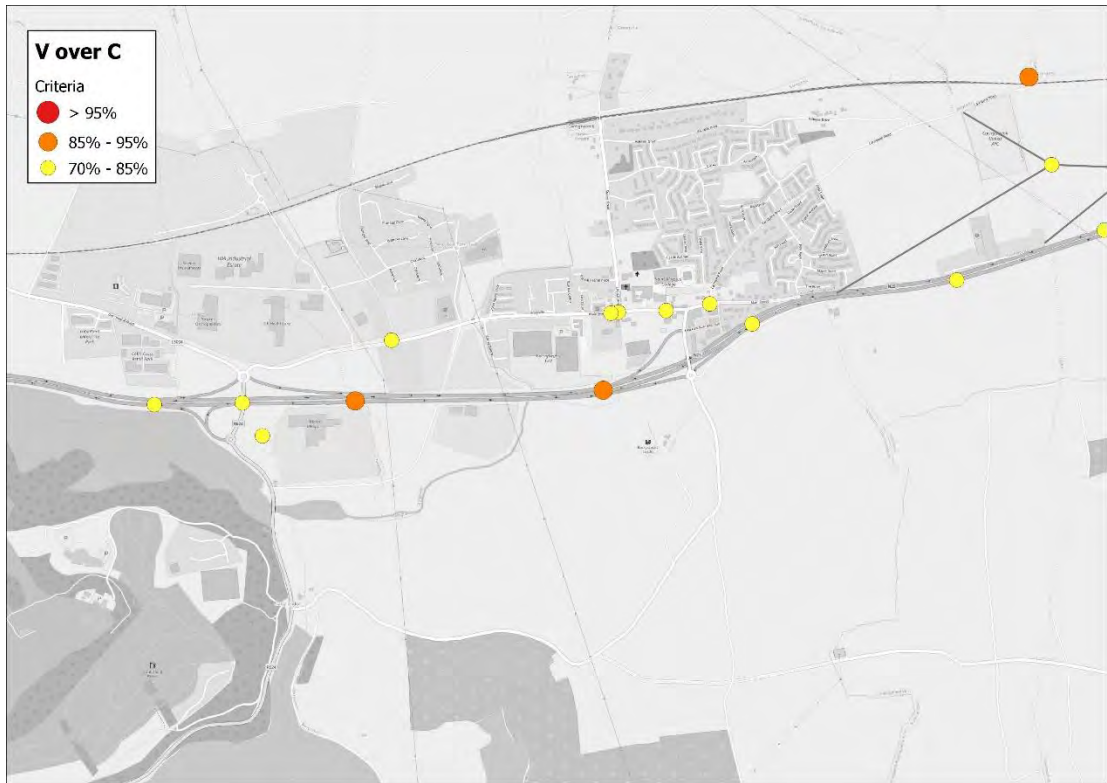
Figure 12 AM V/C Analysis – Rail Sensitivity Carrigtwohill
