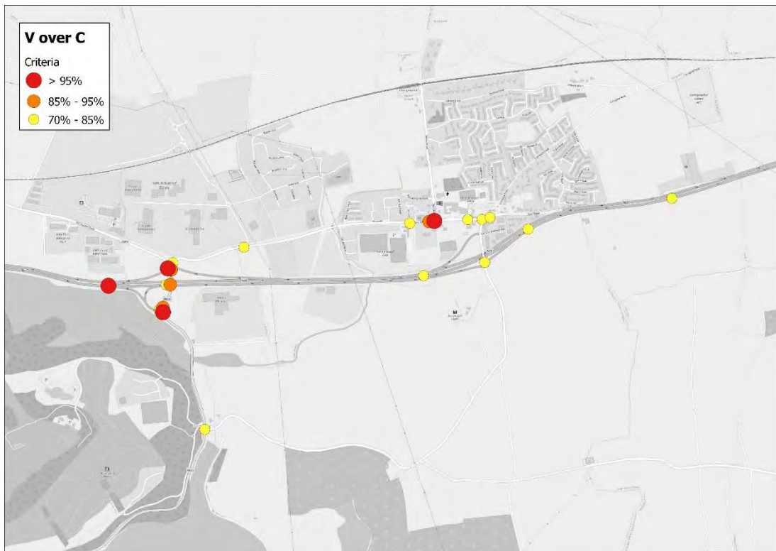
Figure 4 AM V/C Analysis – Rail Test Carrigtwohill
