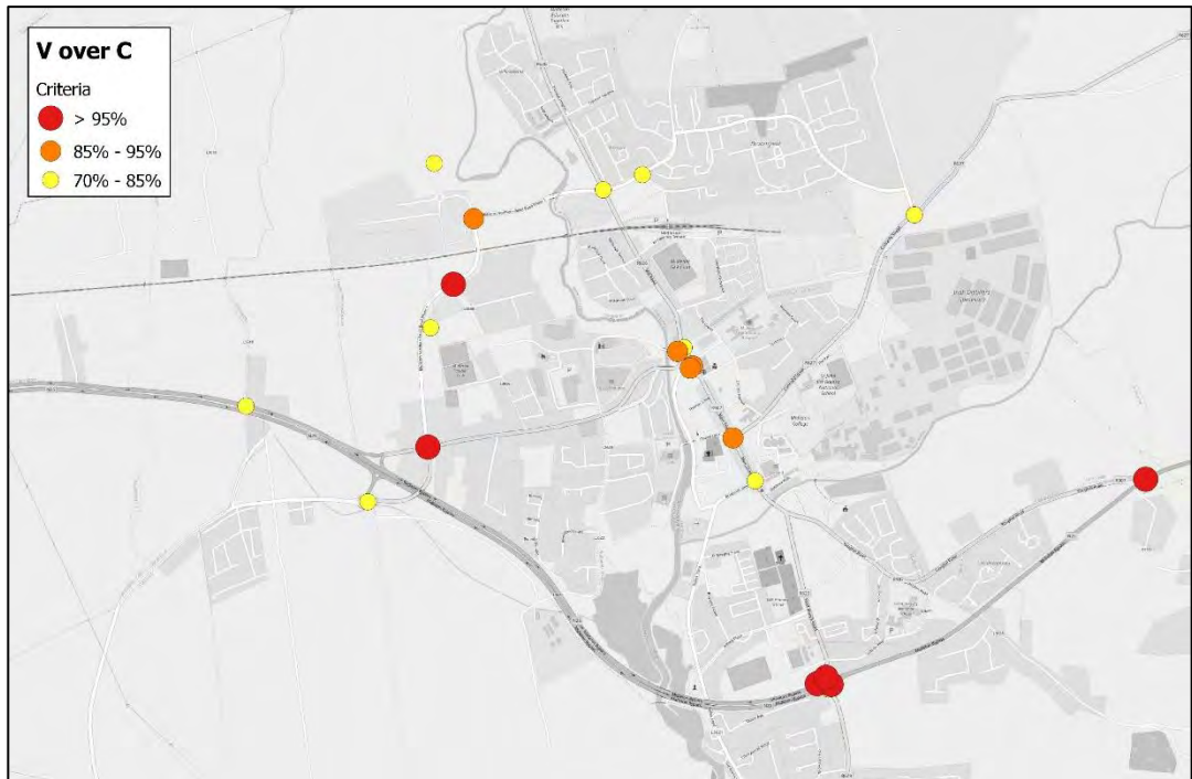
Figure 11-7 PM V/C Analysis – Do-Minimum Carrigtwohill
