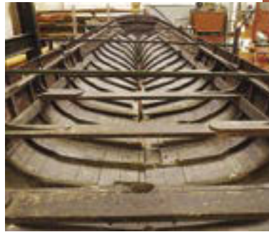
5. An interior view of the after portion of the Bantry Boat showing the damage to her floors and keel. The vessel, which is owned by The National Museum of Ireland and is entirely original, is undergoing an intensive programme of conservation at Merseyside Maritime Museum. She will be put on display in Dublin in 2006.
