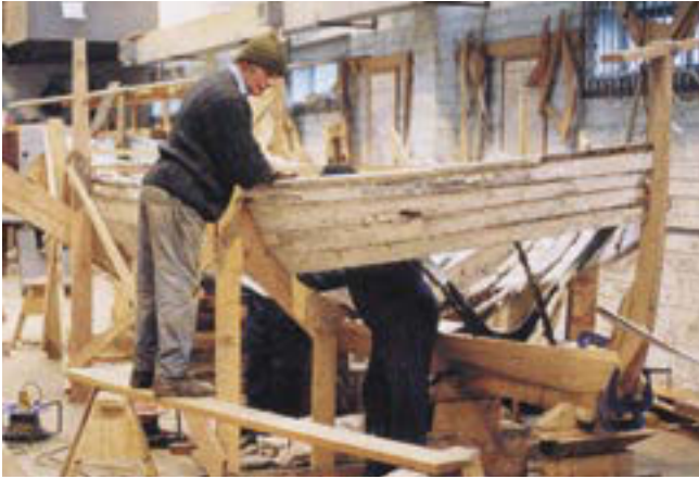
Figure 4. Restoration of an Inishboffin yawl with Anton McBride of Meevagh, Rossguill, Co Donegal, 1998.
