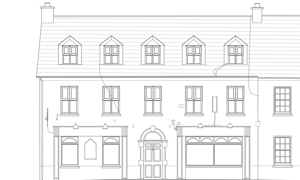
Condition in 2013. Facade altered by the addition of fibreboard shopfront surrounds, PVC windows, roof overhang, wiring and light fittings. This building is now almost unrecognisable as an historic structure.
