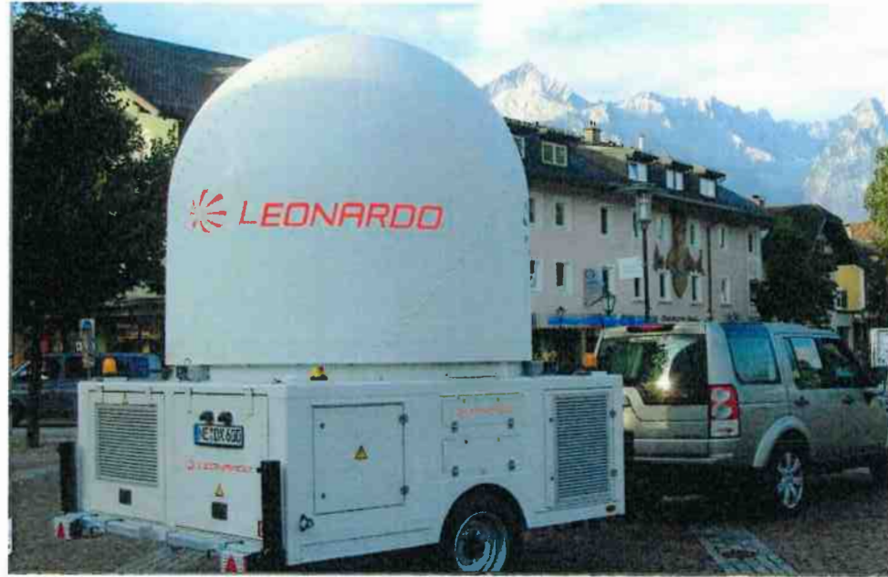
Figure 3 Mobile Radar with Radome Fitted
