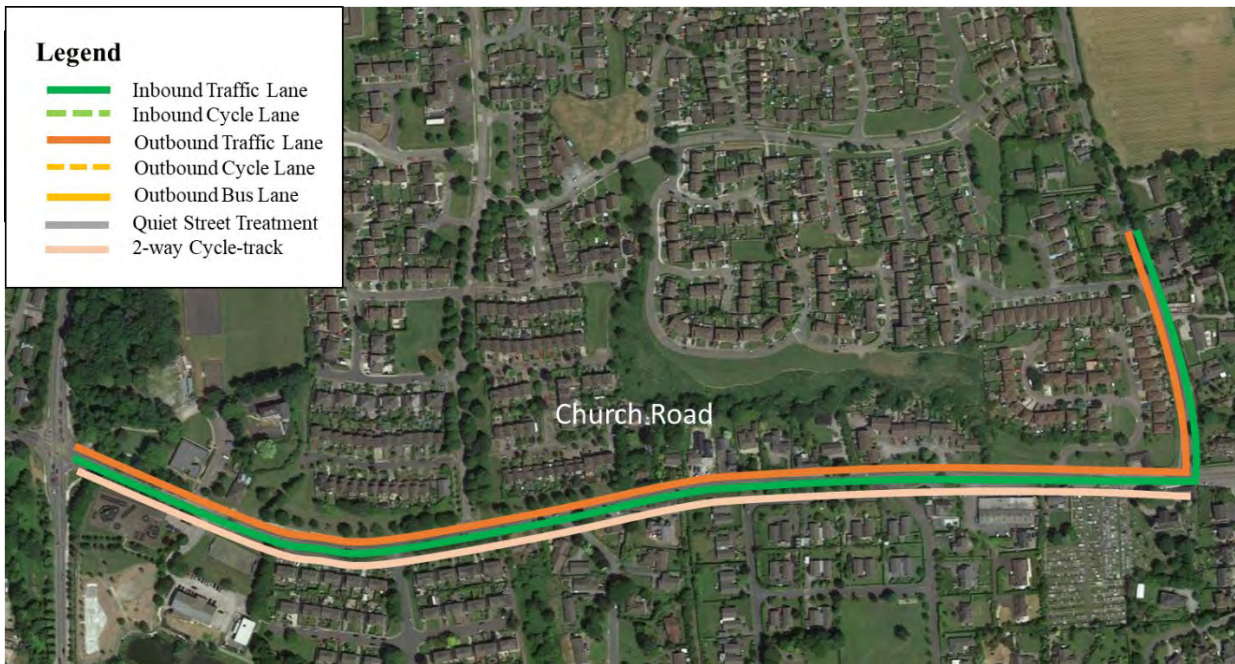
Figure 25 Church Road/Rock Road Option 2 – Infrastructure elements
