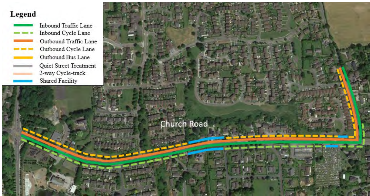
Figure 27 Church Road/Rock Road Option 3 – Infrastructure elements
