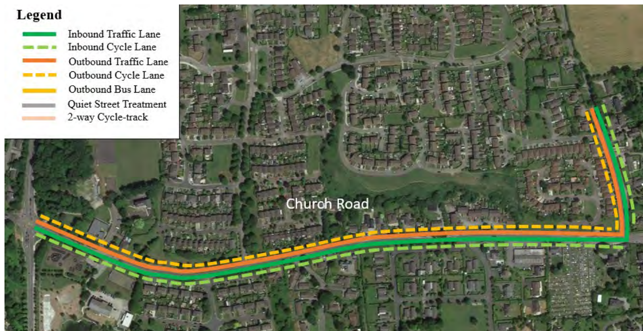
Figure 23 Church Road/Rock Road Option 1 – Infrastructure elements
