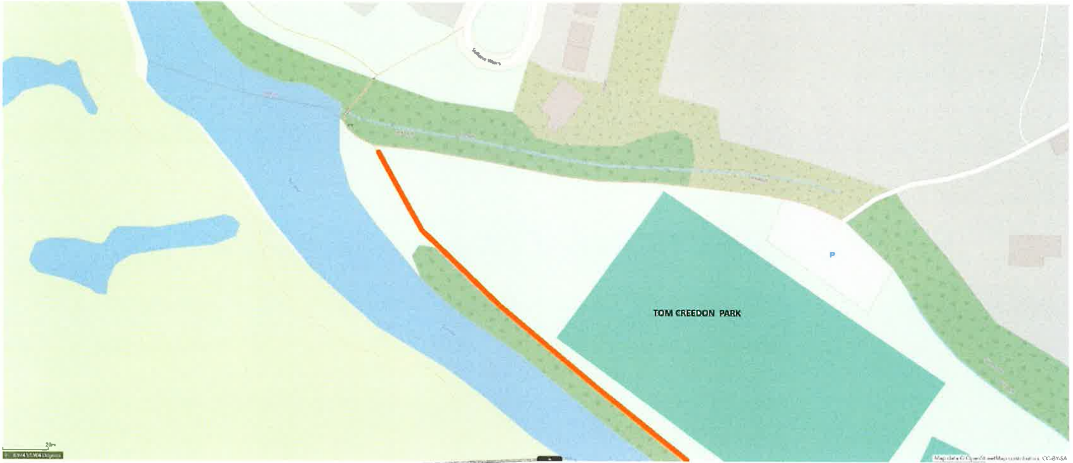
SECTION VIEW OF TOM CRENDON PARK WIDTH OF PATH/CYCLEWAY TO BE INCREASED FROM .9- 1.4M TO 2.9-3.0M
