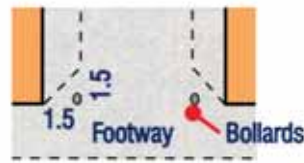
Entrance widened by 1.5m each side
