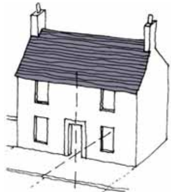
Symmetrical elevation has powerful presence and usefully commands the adjoining space thus tying house and space into one composition
