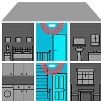
Typical minimum smoke alarm installation
