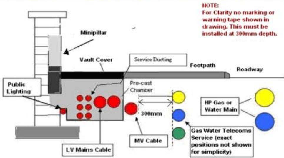
Normal standard clearance = 300mm. Clearance from High Pressure pipes = 600mm
