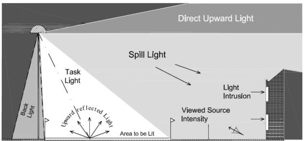
Figure 1 – Types of obtrusive light
