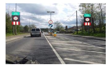
Gateway lighting using supplementary LED lighting on double-headed column in central island. These should be hinged and socketed to allow the column to be lowered for Abnormal Loads
