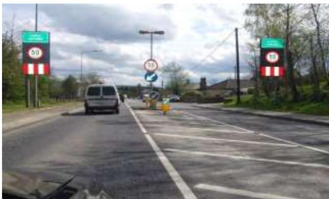
Gateway lighting using supplementary LED lighting on double-headed column in central island. These should be hinged and socketed to allow the column to be lowered for Abnormal Loads
