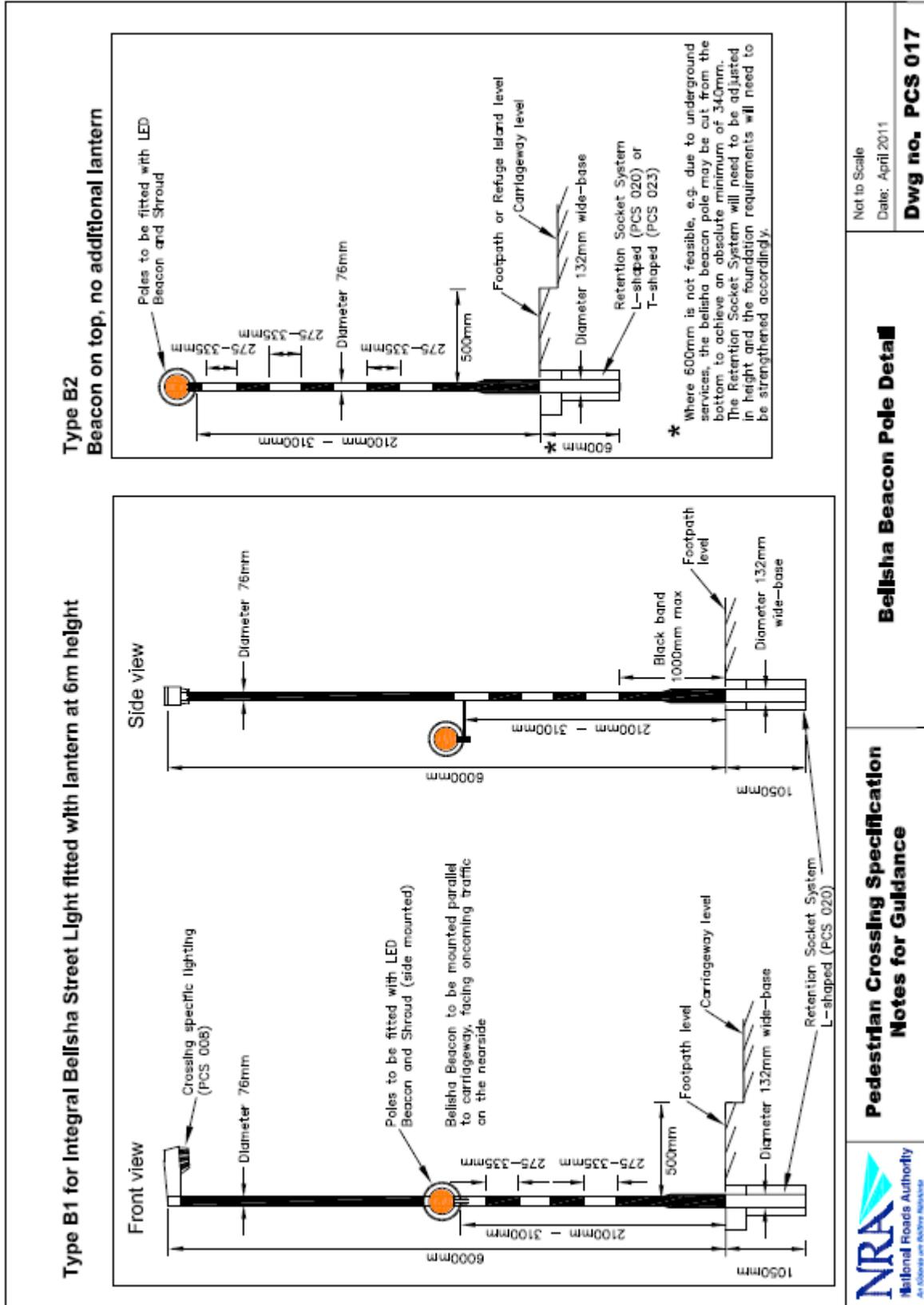
Figure 19: Retention Socket System for Zebra Crossing
