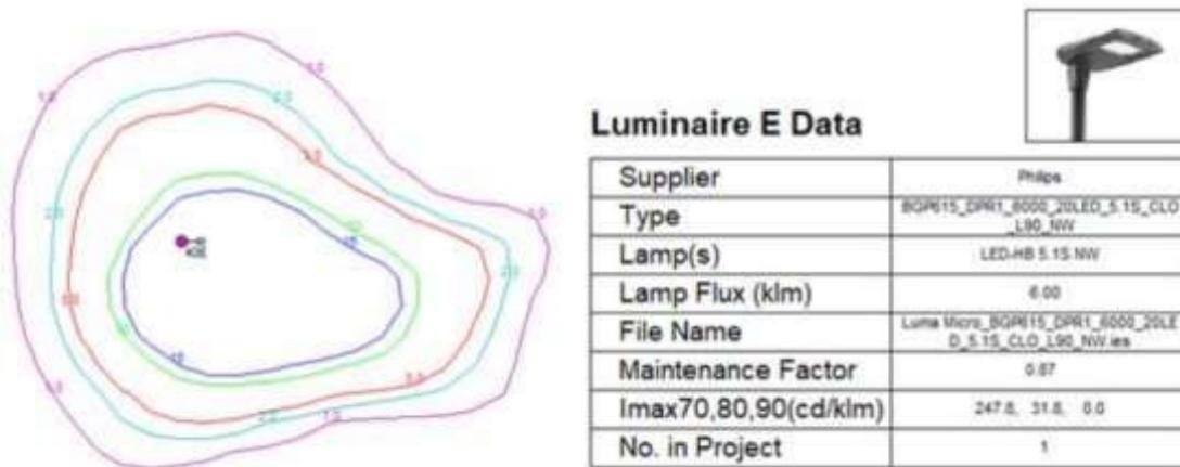
**For a pole on the Right use a Left optic. BGP615\_DPL1\_6000\_20LED\_5.1S\_CLO\_L90\_NW\_PT – NO DIMMING**
