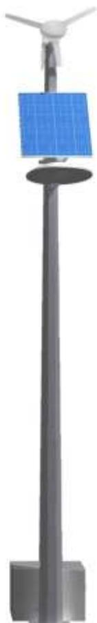
**Construction:** Typically an 8m flanged octagonal pole with turbine, solar panel and luminaire. Batteries are stored in a separate box at base of pole.
