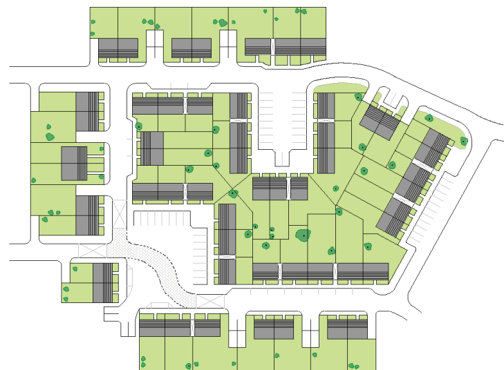
Figure 3.1 Short, wide spaces with parking in front of houses, within limited width street networks
