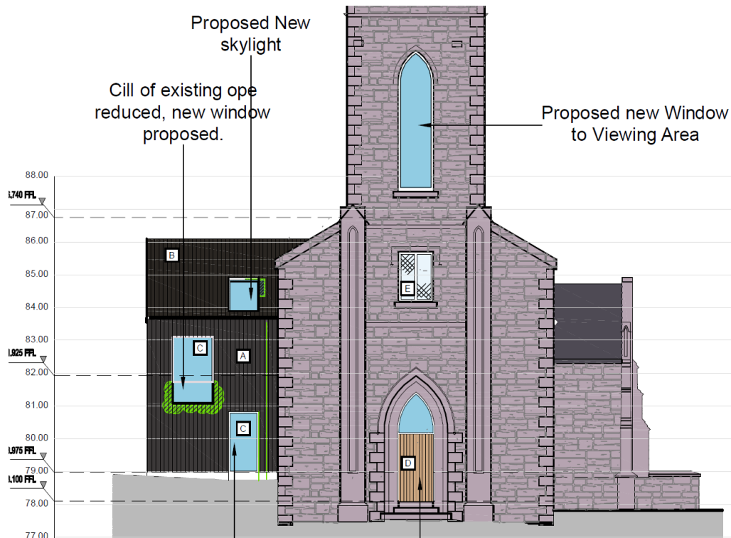
Proposed contemporary burnt larch cladding to walls and roof of existing extension
