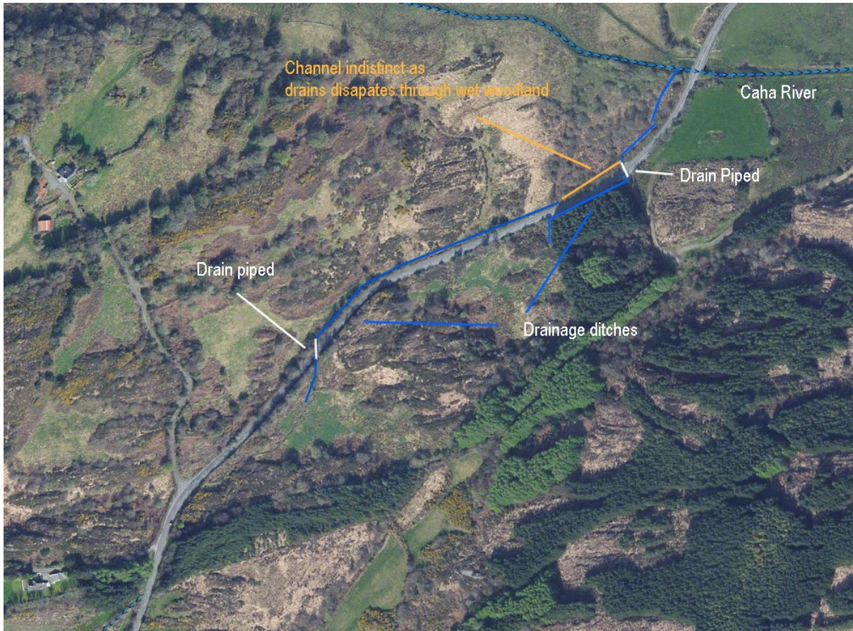
Figure 5. Drainage channels at proposed development site
