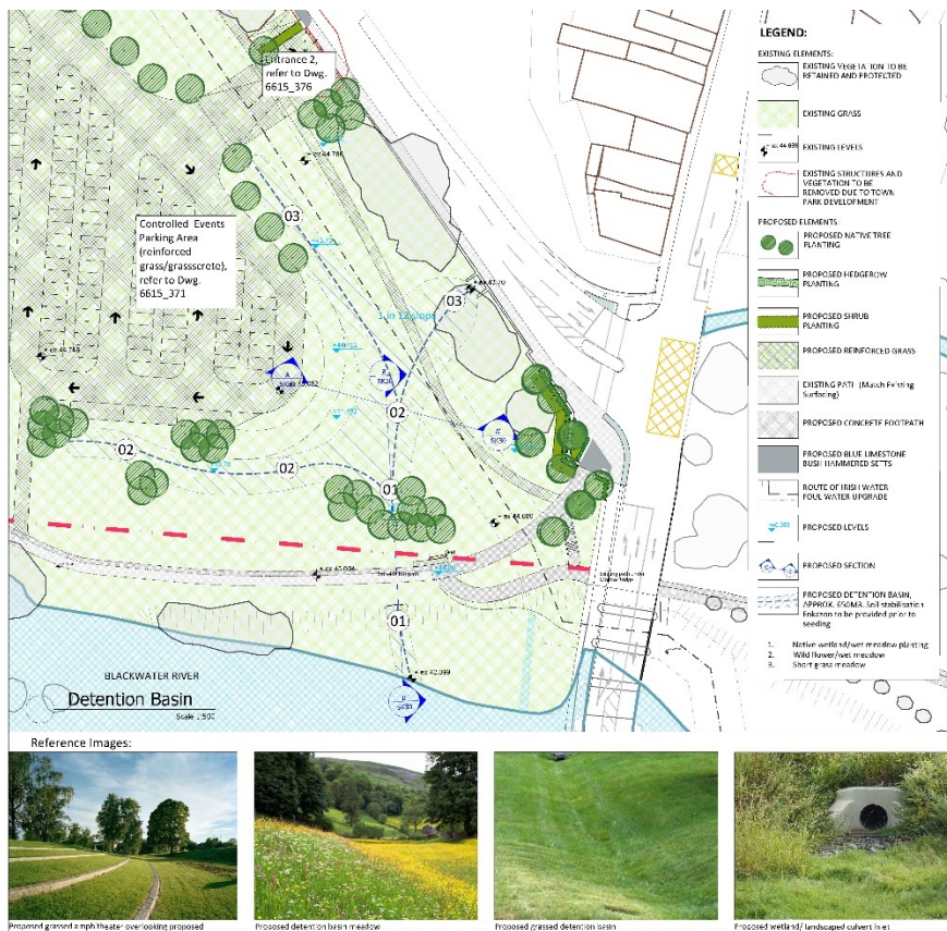
Figure 46 Vegetated swale and detention basin area
