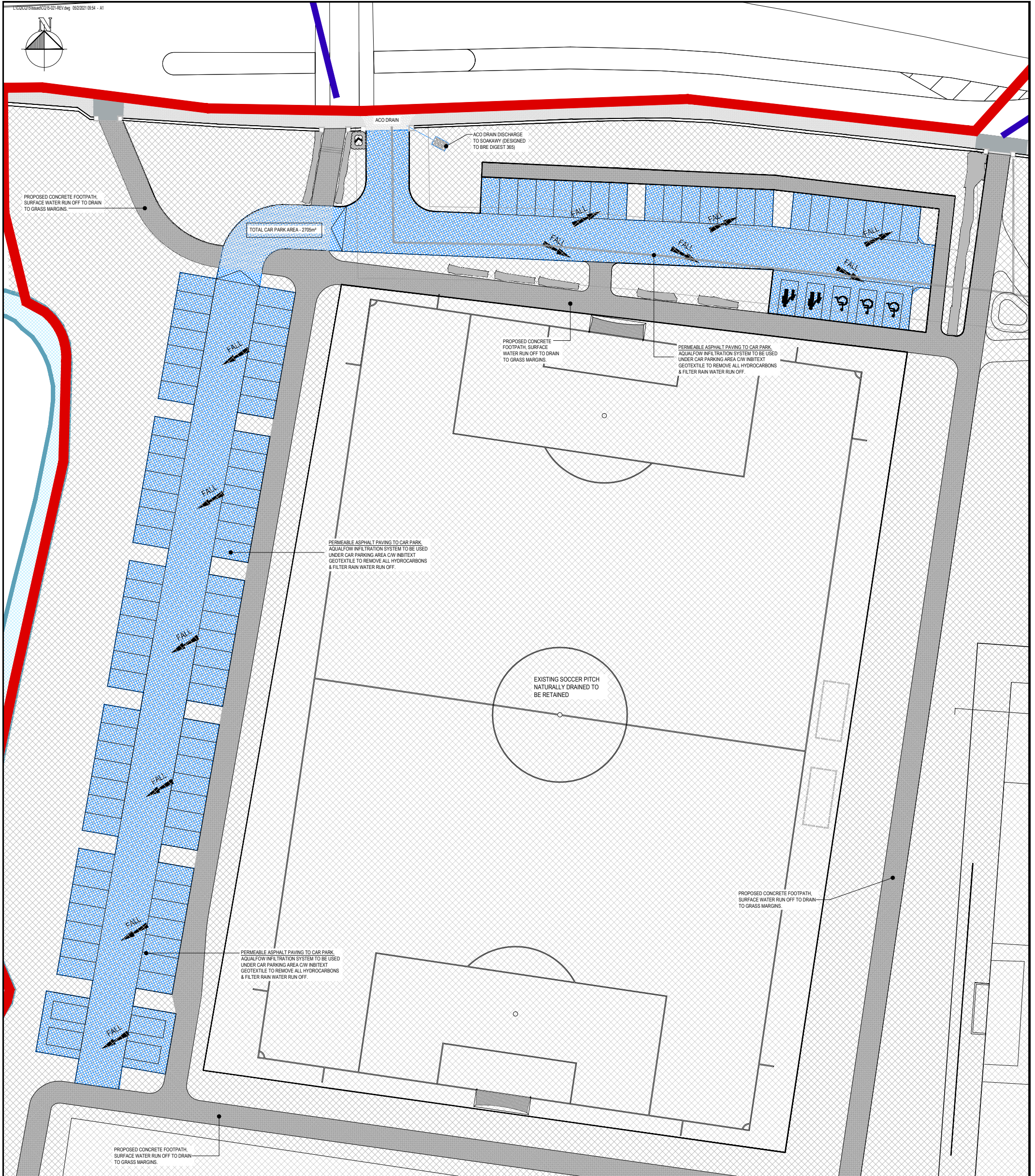
PROPOSED STORM WATER LAYOUT TO NEW CAR PARK SCALE 1:250
