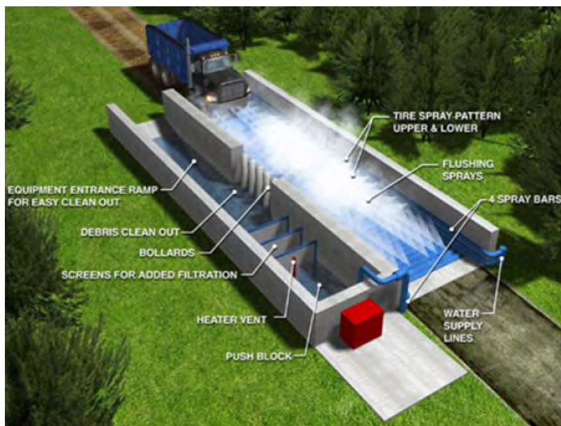
Figure 12 – Example of wheel washing facility to be provide byut the contractor for the duration of the site works
