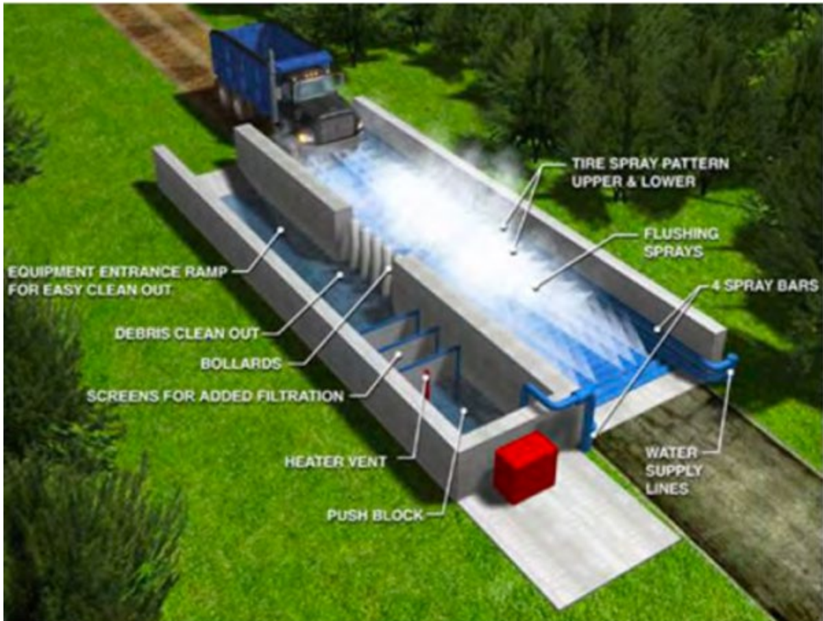
Figure 22. Example of wheel washing facility to be provide byut the contractor for the duration of the site works
