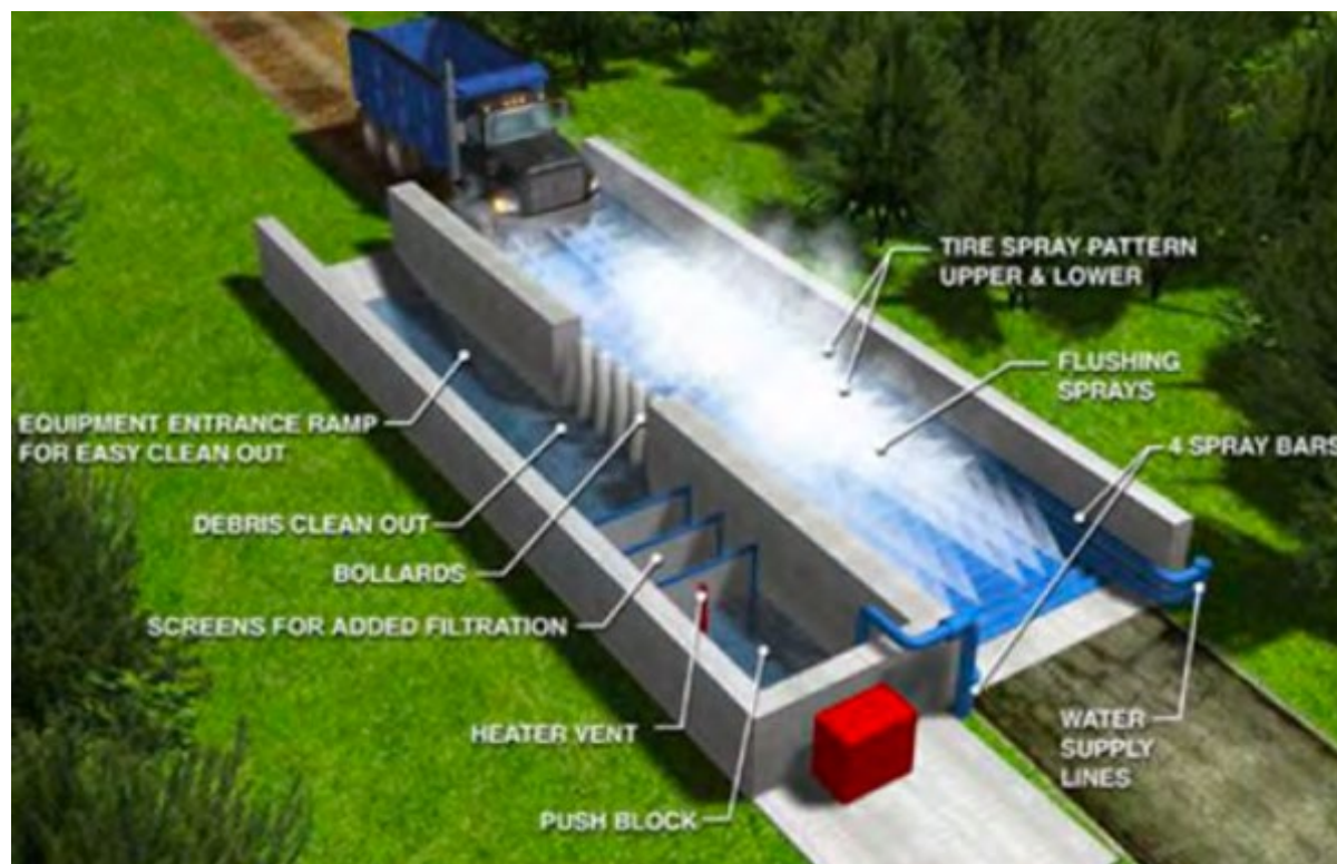
Figure 6-2 Example of wheel washing facility to be provide by the contractor for the duration of the site work
