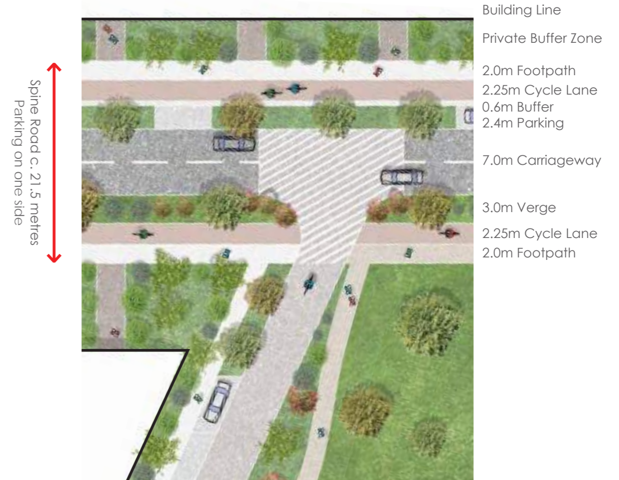
Partial Plan of spine road, showing potential junction between spine road and a local access road
