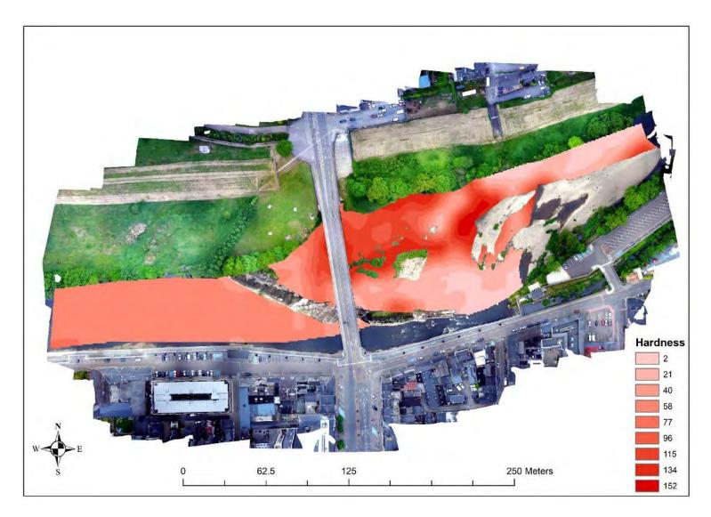
Figure 3.3 Relative river bed hardness map of the survey area, July 2020 (darker shading indicates softer substrata)
