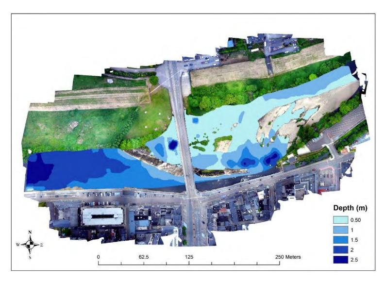
Figure 3.2 Bathymetry map of the survey area, July 2020 (darker shading indicates deeper water)
