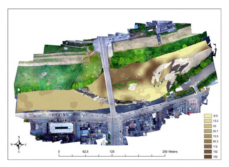
Figure 3.4 Relative river bed rugosity (roughness) map of the survey area, July 2020 (darker shading indicates areas of smoother substrate complexity)
