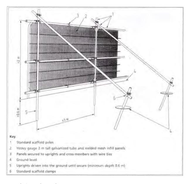
Fig.1 Default Specification for Protective Barrier
