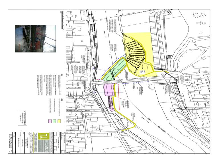
Figure 4. Phasing of instream works | Source T.J. O'CONNOR & ASSOCIATES
