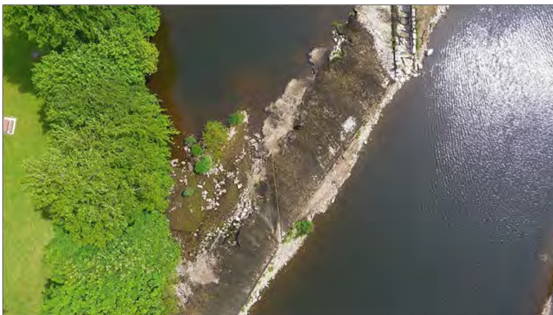
Plate 13 Aerial photograph showing the western extreme of the pier, with paved area shown in the acute angle formed by the weir and northern bank.
