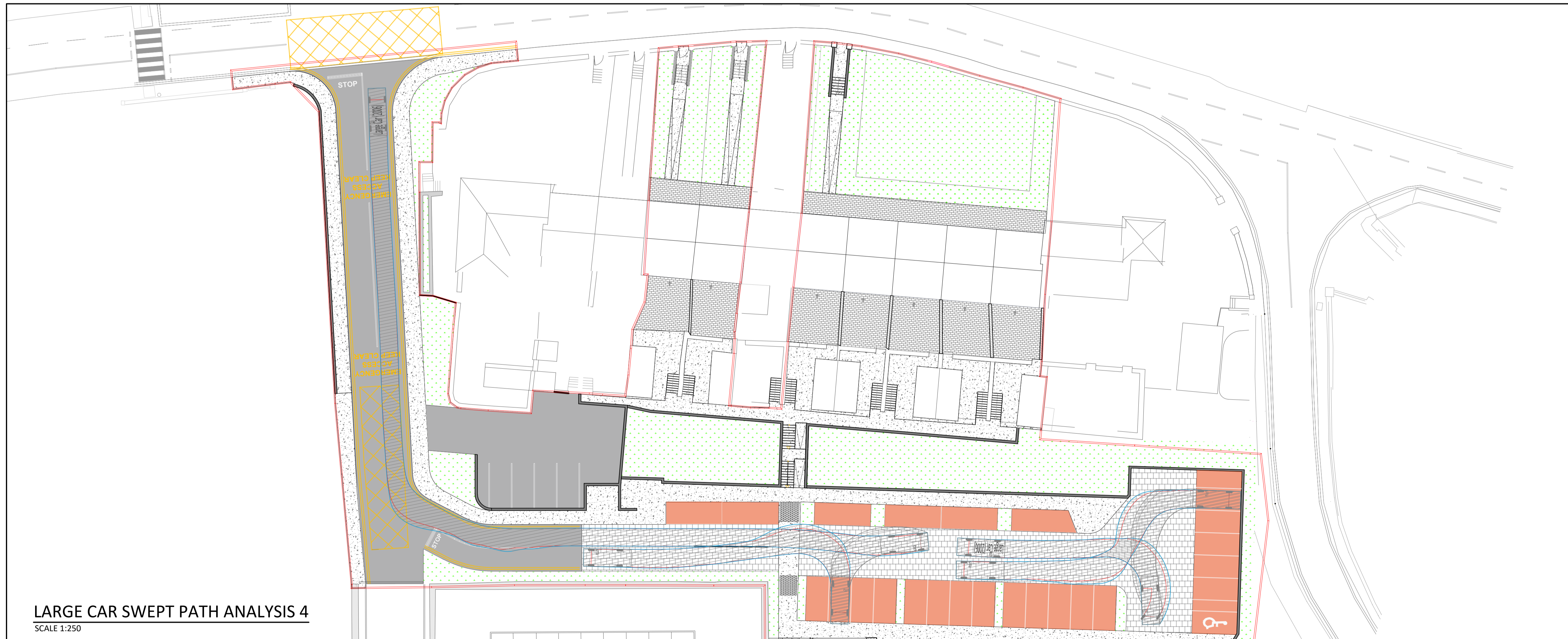
LARGE CAR SWEPT PATH ANALYSIS 3 SCALE 1:200
