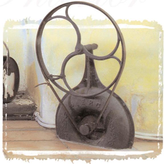
Figure 20. Cast-iron bellows, Ballymacoda. CCC No 161.
