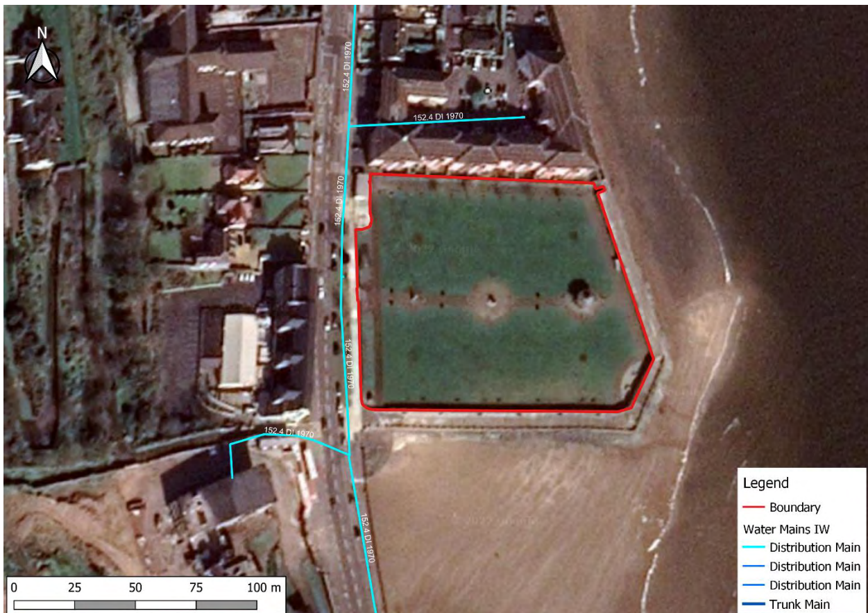
Figure 4-1: Existing watermain surrounding the site
