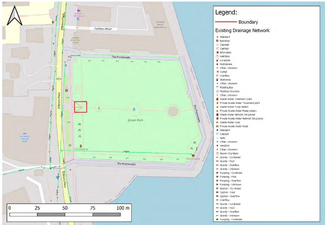
Figure 3-3: Existing Stormwater drainage in the vicinity of the site
