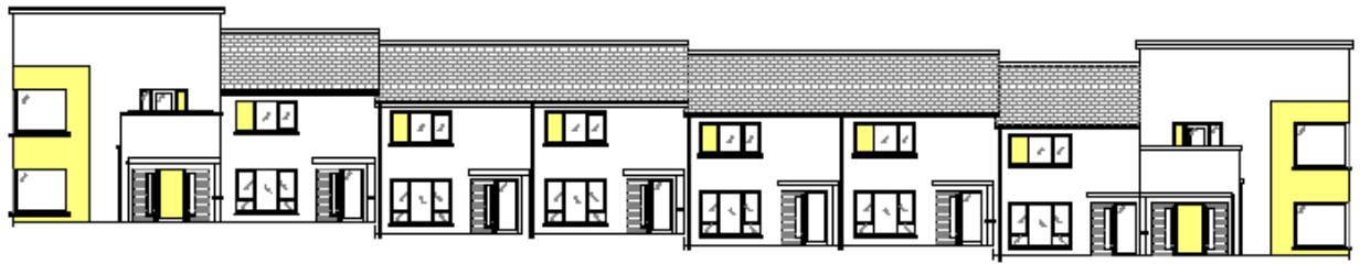
Terrace No.4: Proposed Front Elevation showing 6 No. 2 bed dwellings with 'bookend' 1 bed apartments.
