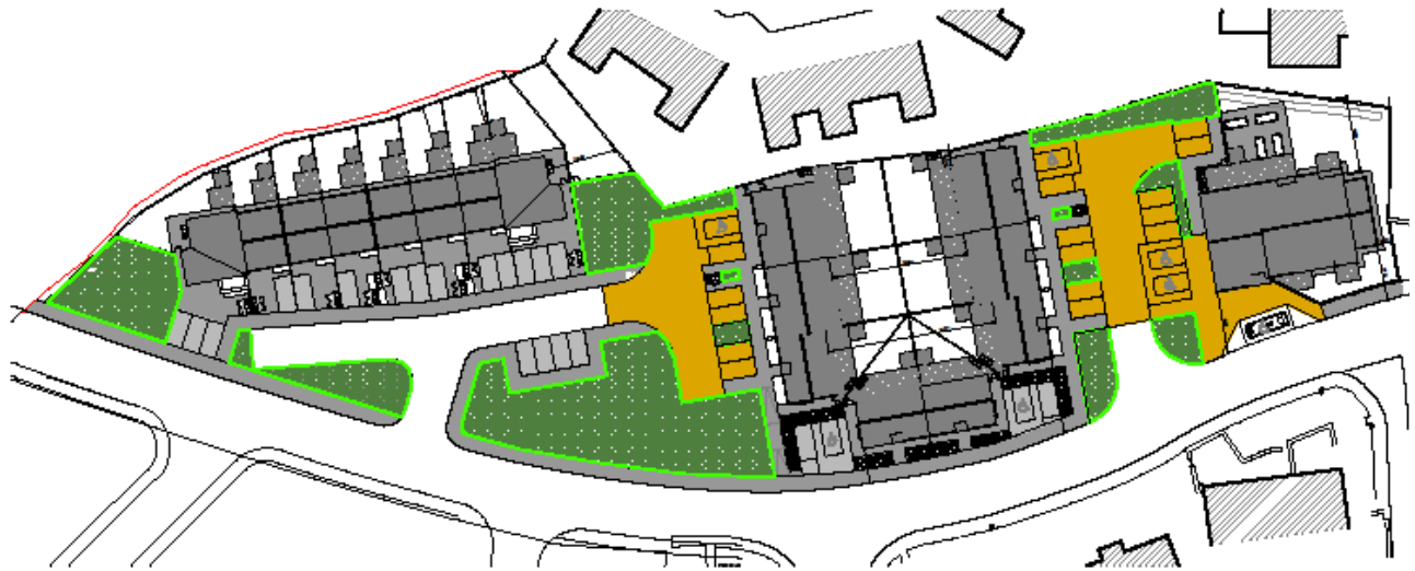
Image of proposed site plan, with public green areas indicated in green and paved homezones
