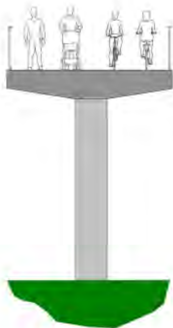
PRECAST CONCRETE DECK AND CONCRETE MONO PILES
