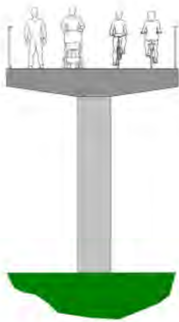
PRECAST CONCRETE DECK AND CONCRETE MONO PILES
