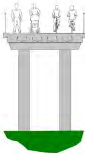
PRECAST CONCRETE DECK AND DOUBLE CONCRETE PIERS WITH CROSSHEAD
