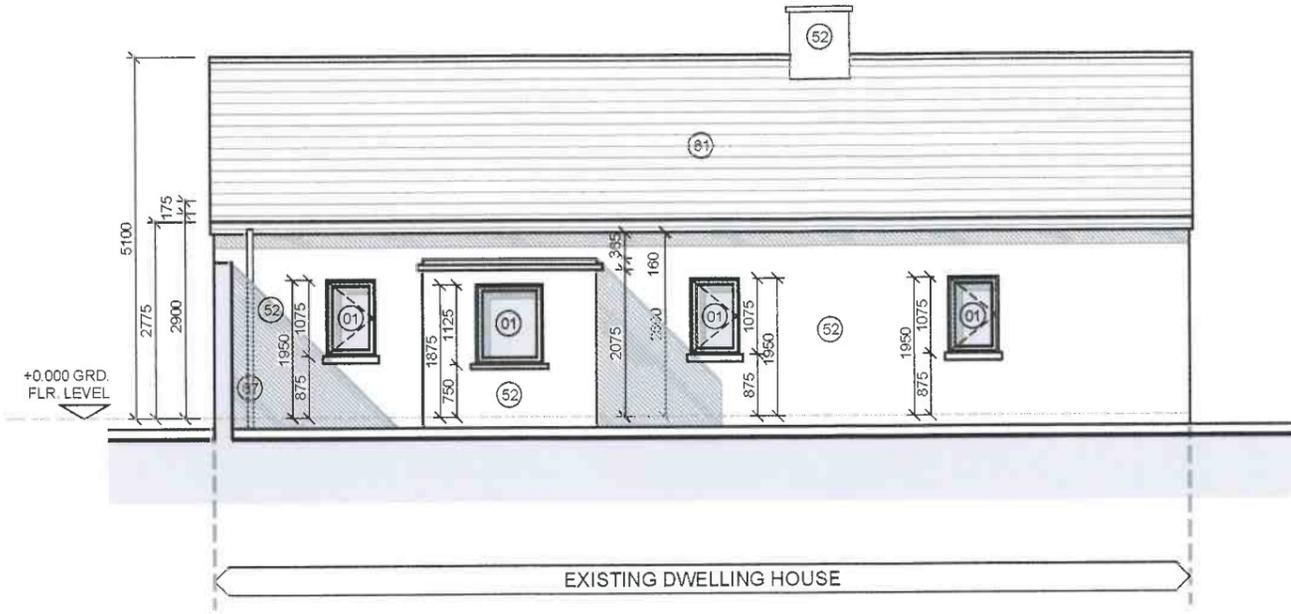
**PROPOSED EAST ELEVATION [ FRONT ELEVATION ]**
