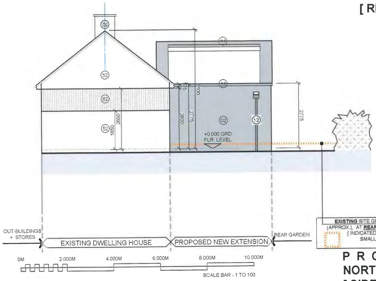
**PROPOSED NORTH ELEVATION [ SIDE ELEVATION ]**
