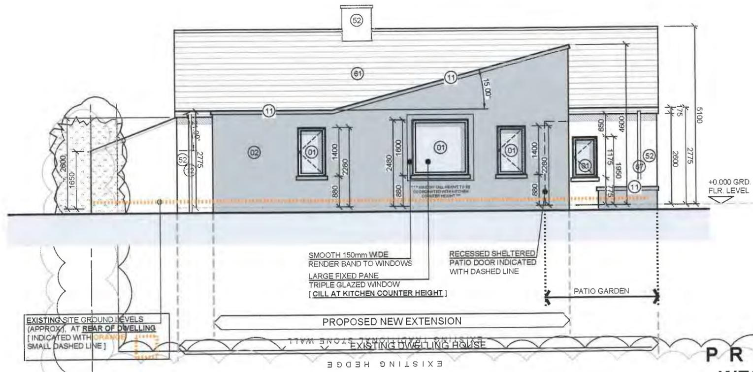
**PROPOSED WEST ELEVATION [ REAR ELEVATION ]**
