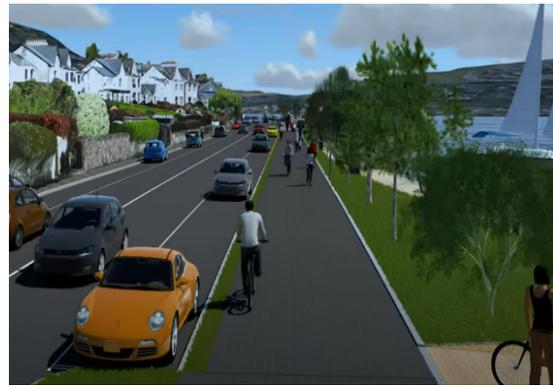
AADT of the order of 3,500 vehicles. These characteristics indicate that the most appropriate form of provision is a segregated facility. As such the proposed design has been developed as an off-road shared use pedestrian and cyclist facilities.
