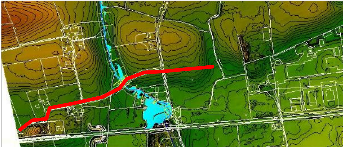
Figure 3-5: Flood Extent for Water Rock 1%AEP
