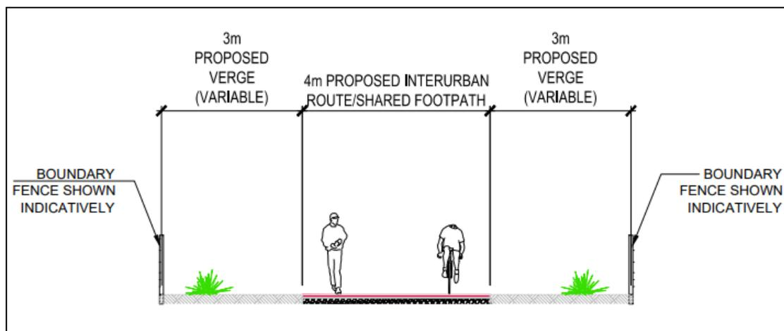
**Figure 3-3 - Typical cross-section of the proposed cycling and walking facility.**
