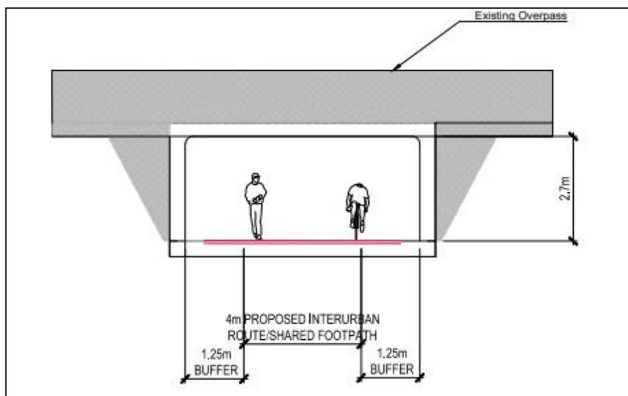
**Figure 3-2 - Typical cross-section through the proposed underpass.**
