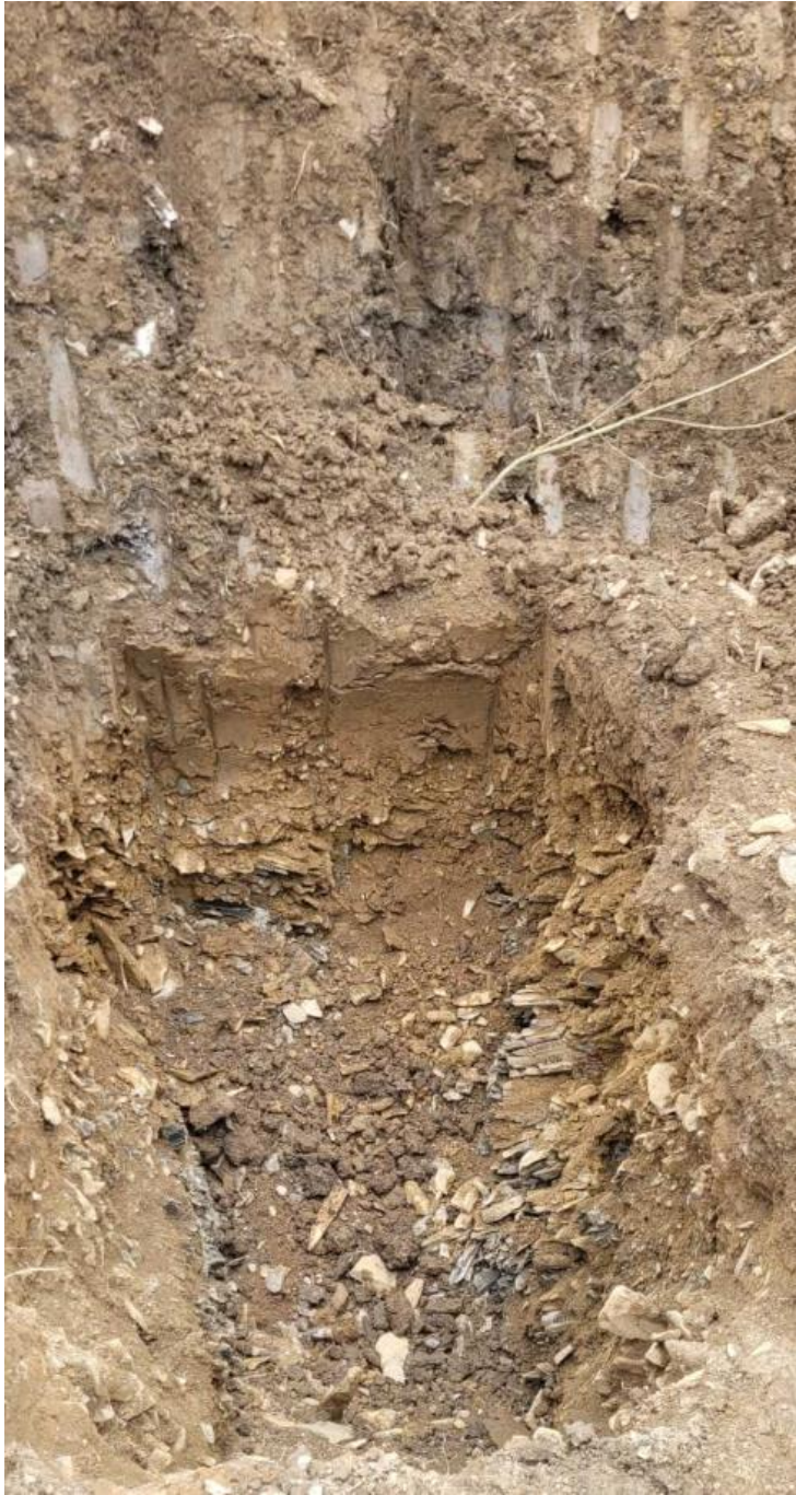
Trial hole to rear of site for no. 19 showing angular GRAVEL / weathered SILTSTONE (shale)
