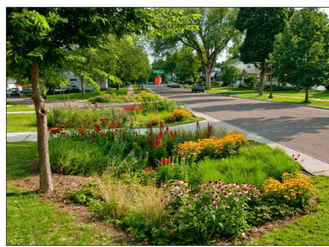
5. Example of raingarden bio swale.
