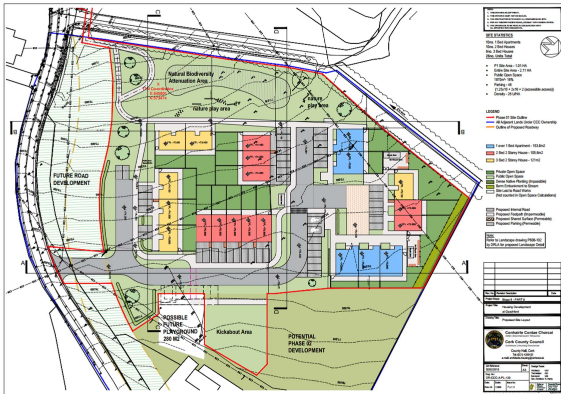
Figure 3: Architect's Site Layout
