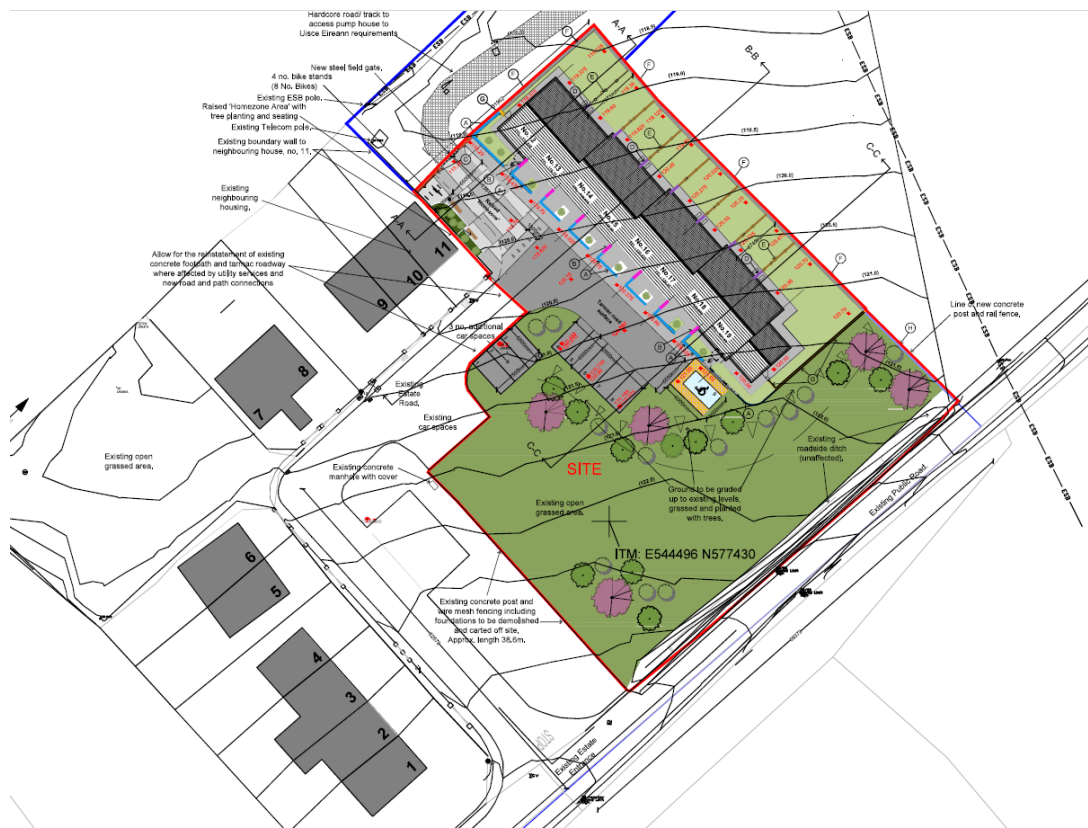
Figure 13 - Proposed site layout plans showing new development and new development in the context of the existing
