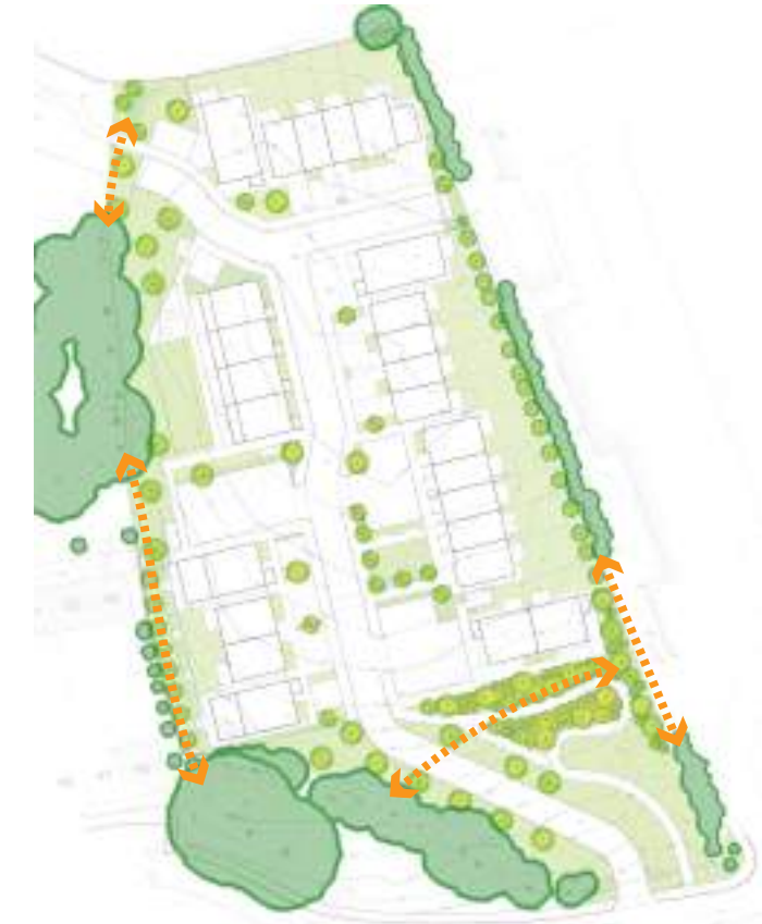
Diagram highlighting the existing peripheral trees (dark green) with proposed tree planting links (orange lines).
