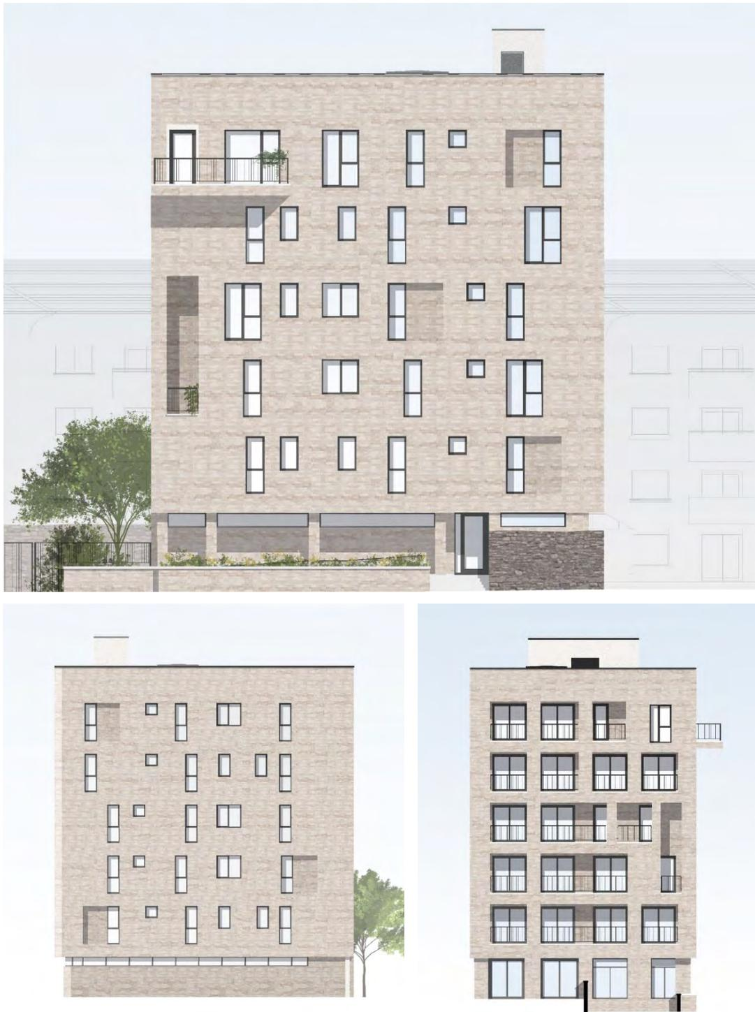
*Figure 23. Elevations showing material palette of buff brick, existing rubble stone, steel railings, aluminium windows ( top: south elevation-from public car park, bottom left: north elevation- from existing apartment complex, bottom right: west elevation- from walled garden)*
