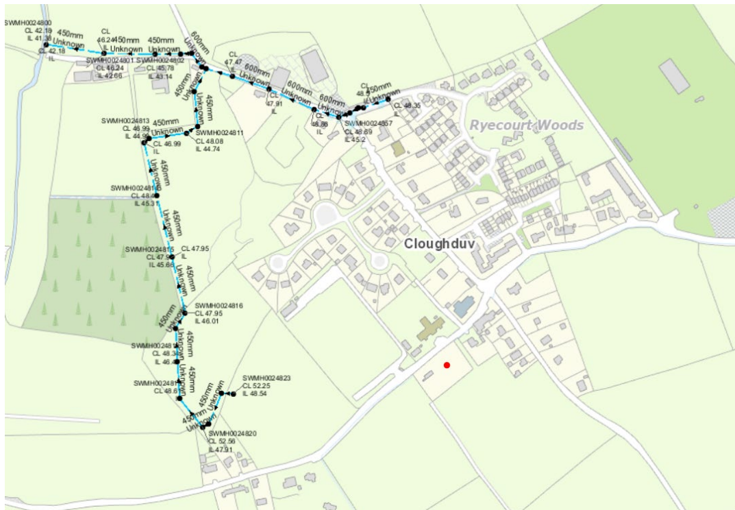
Figure 15. Layout of existing stormwater network in Cloughduv.
