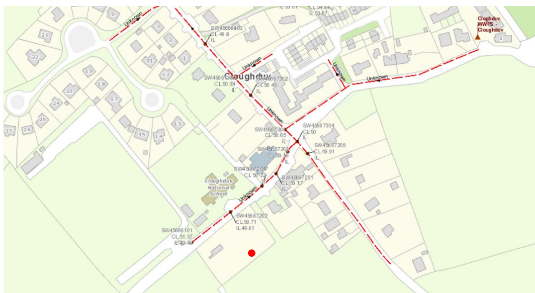
Figure 14. Layout of existing foul network in Cloughduv.
